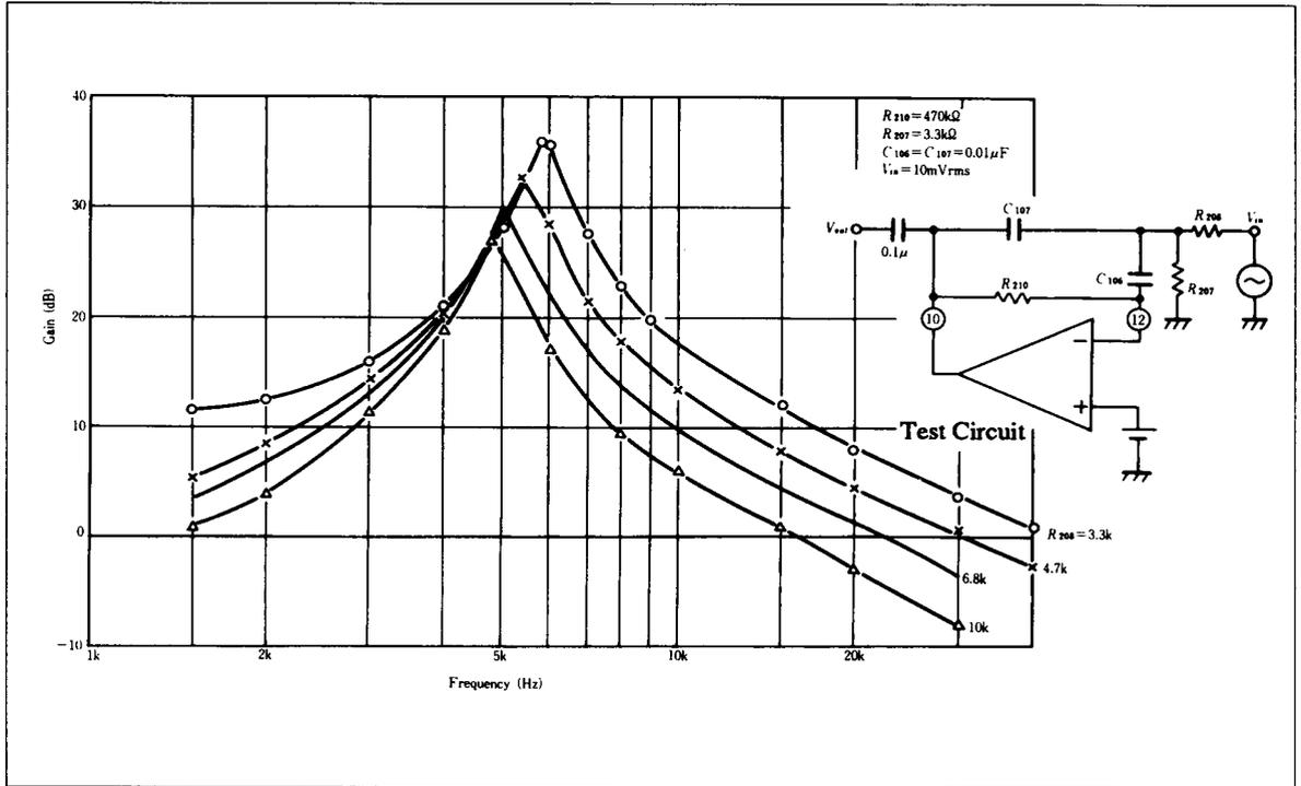
Filter Amplifier Frequency Characteristics
