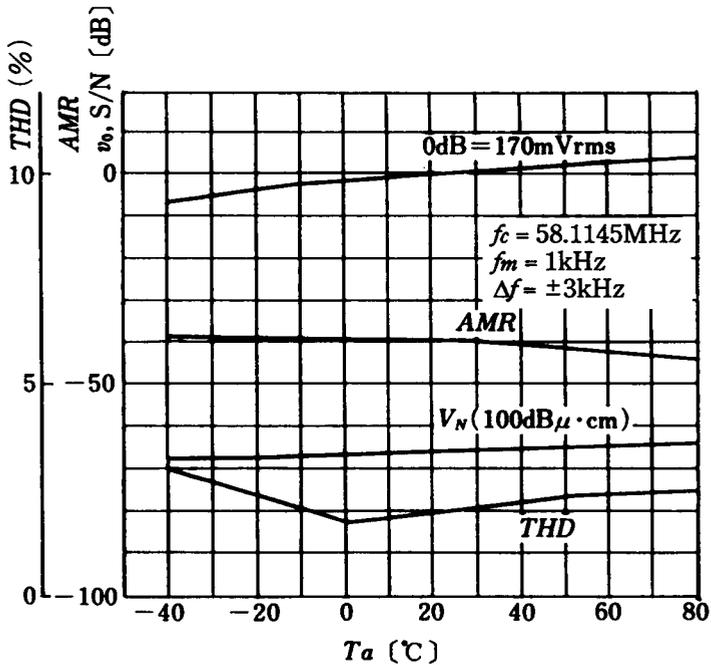
Converter Gain-Temperature Characteristics
