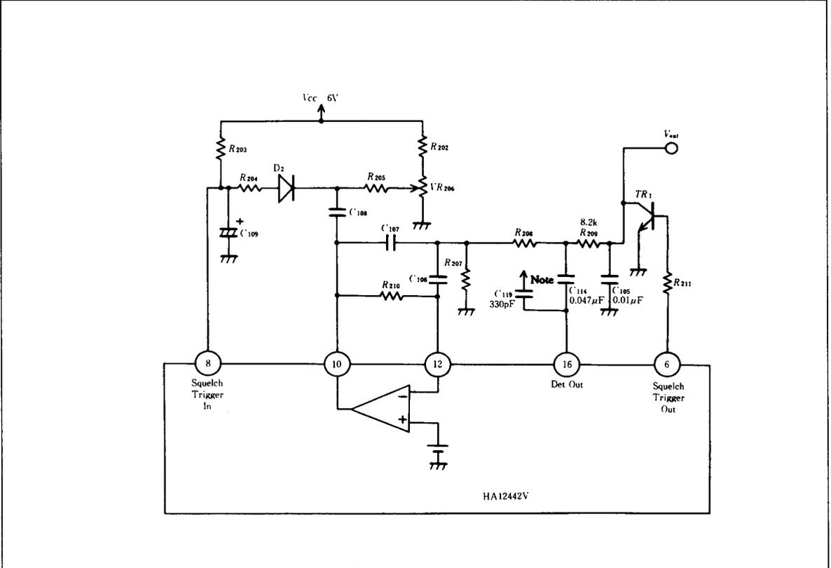
Note: Connect C119 to Vcc line as near to pin 13 as possible.
