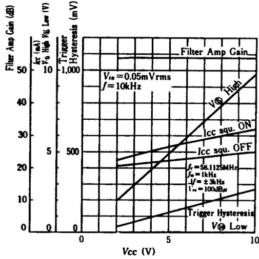
Input Sensitivity-Supply Voltage Characteristics
