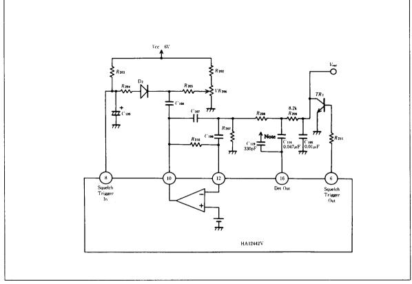
Note: Connect C119 to Vcc line as near to pin 13 as possible.
