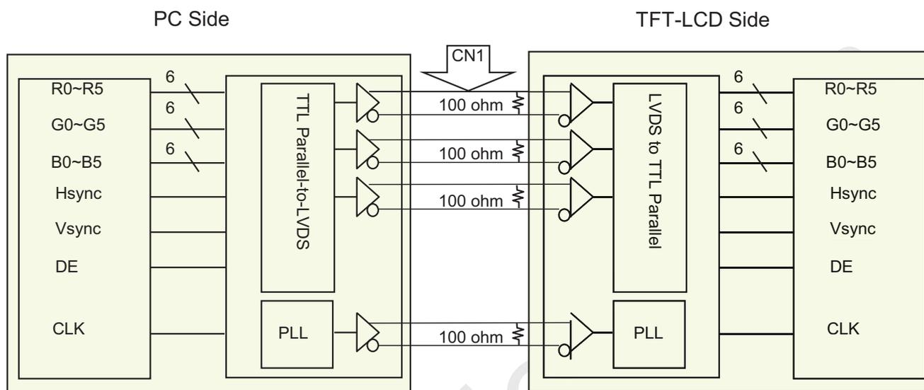
Note. Transmitter : Thine THC63LVDM63A or equivalent.
