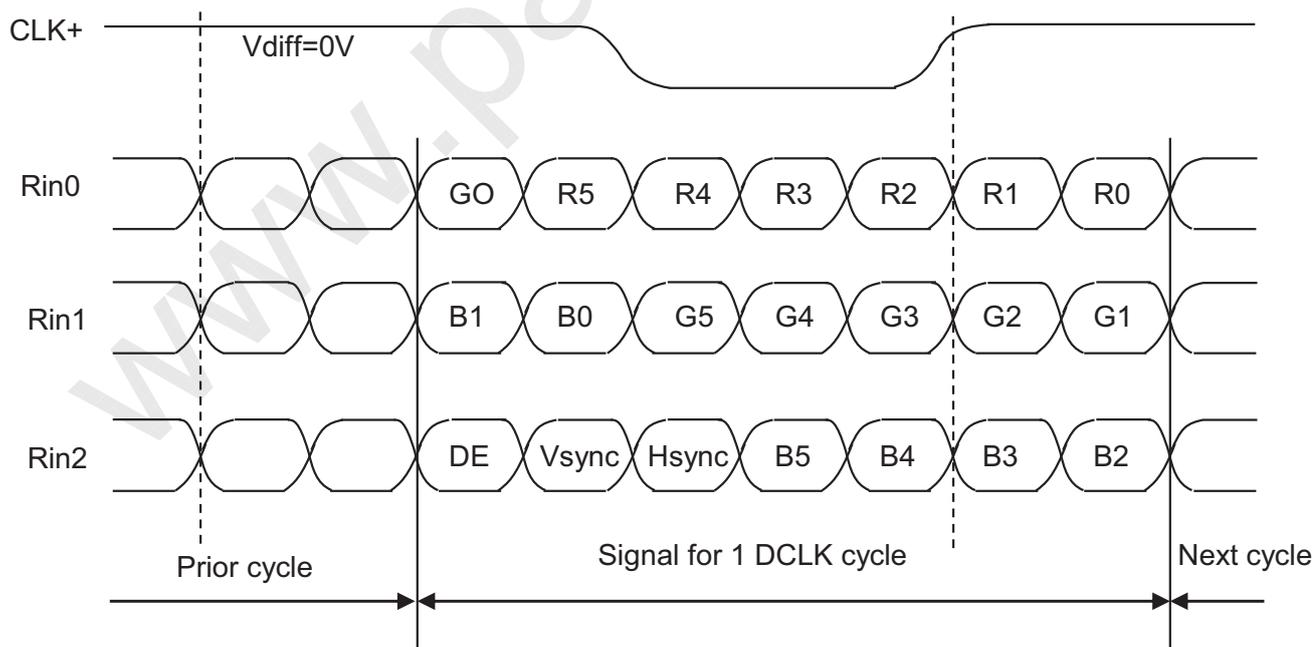
Note. Pin connection in case of using Thine THC63LVDM63A
