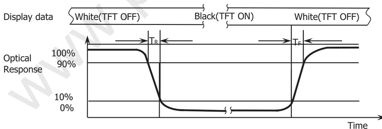
The electro-optical response time measurements shall be made as shown in FIGURE 4 by switching the "data" input signal ON and OFF. The times needed for the luminance to change from 10% to 90% is  $T_d$  and 90% to 10% is  $T_r$ .
