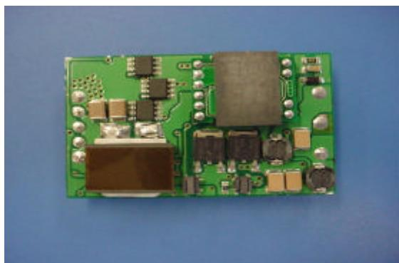
**The HBQ SERIES** is a new line of isolated DC/DC converters in the industry standard quarter brick format.
