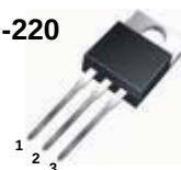
1.Gate 2. Drain 3. Source
