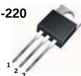
1.Gate 2. Drain 3. Source
