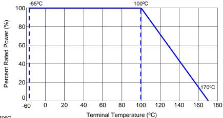
Operating temperature range of -55 to 170°C. Storage condition: 5~35°C, humidity of 40~75%.
