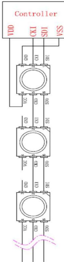
In the practical application circuit, the signal input and output pins of the IC signal input and output pins should be connected to the signal input and output terminals. In addition, in order to make the IC chip is more stable, even the capacitance between beads is essential back;
