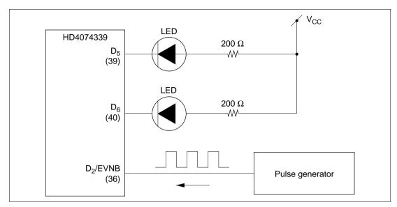
Figure 24-5 Frequency Determination Block Circuit Diagram
