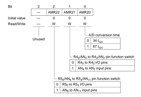
Bit 2—R5<sub>0</sub>/AN<sub>8</sub> to R5<sub>3</sub>/AN<sub>11</sub> Pin Function Switch (AMR22): Selects whether the R5<sub>0</sub>/AN<sub>8</sub> to R5<sub>3</sub>/AN<sub>11</sub> pins function as the R5<sub>0</sub> to R5<sub>3</sub> I/O pins or as the A/D converter channel 8 to 11 input pins (AN<sub>8</sub> to AN<sub>11</sub>).
