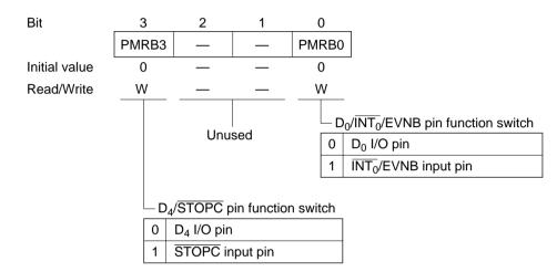
**Bit 3—D\_4/\overline{\text{STOPC}} Pin Function Switch (PMRB3):** Selects whether the  $D_4/\overline{\text{STOPC}}$  pin is used as the  $D_4$  I/O pin or as the stop mode clear pin (STOPC).
