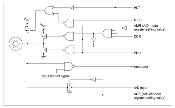
Figure 8-3 R Port/Analog Input Shared Function Pin Circuit
