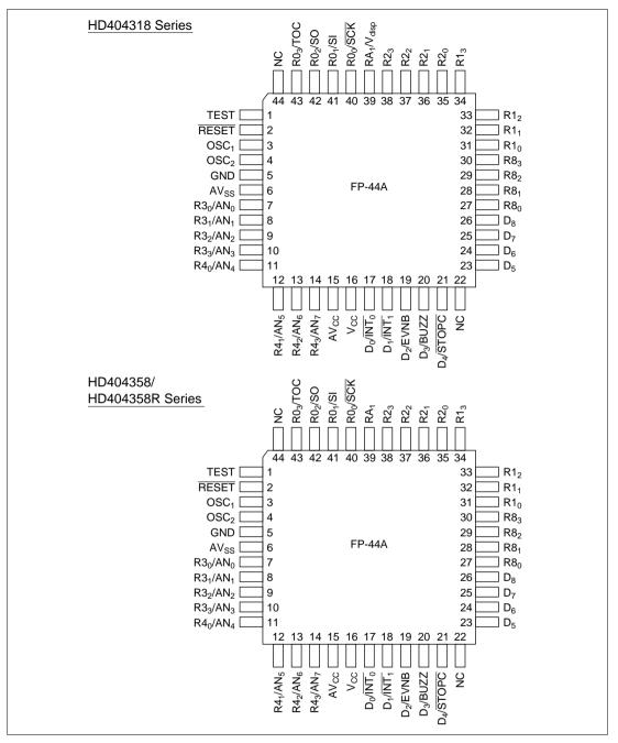
Figure 1-12 HD404318, HD404358 and HD404358R Series Pin Arrangements (FP-44A Package: Top View)
