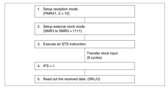
Figure 20-9 Data Reception Procedure (External Clock Mode)
