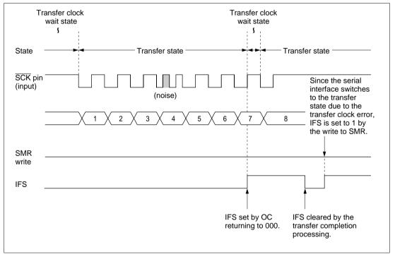
Figure 20-17 Transfer Clock Error Detection Sequence
