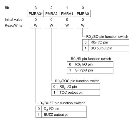
Note: \* Applies to the HD404318, HD404358, HD404358R, HD404339, and HD404369 Series. The PMRA3 bit is unused in the HD404344R and HD404394 Series.
