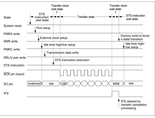
Figure 20-6 Serial Transmission Operation Sequence (External Clock Mode)
