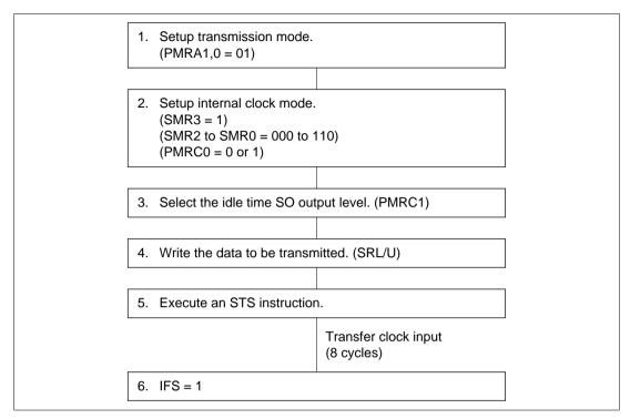
Figure 20-7 Data Transmission Procedure (Internal Clock Mode)
