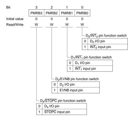
Bit 2— $D_2$ /EVNB Pin Function Switch (PMRB2): Selects whether the  $D_2$ /EVNB pin functions as the  $D_2$  I/O pin or as the timer B event input pin (EVNB).
