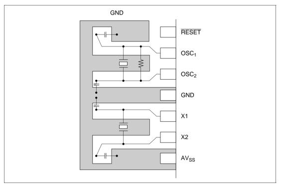
Figure 14-2 Wiring Example for Crystal and Ceramic Oscillators
