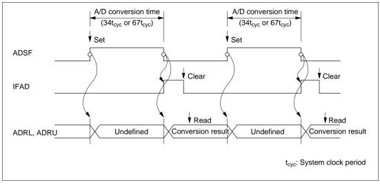
Figure 15-3 A/D Converter Operation Timing Chart
