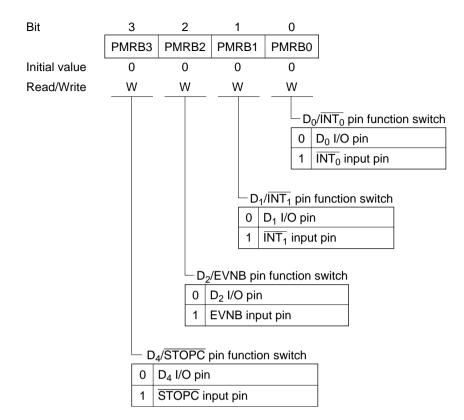
**Bit 3—D<sub>4</sub>/STOPC Pin Function Switch (PMRB3):** Selects whether the  $D_4/\overline{\text{STOPC}}$  pin is used as the  $D_4$  I/O pin or as the STOPC input pin.
