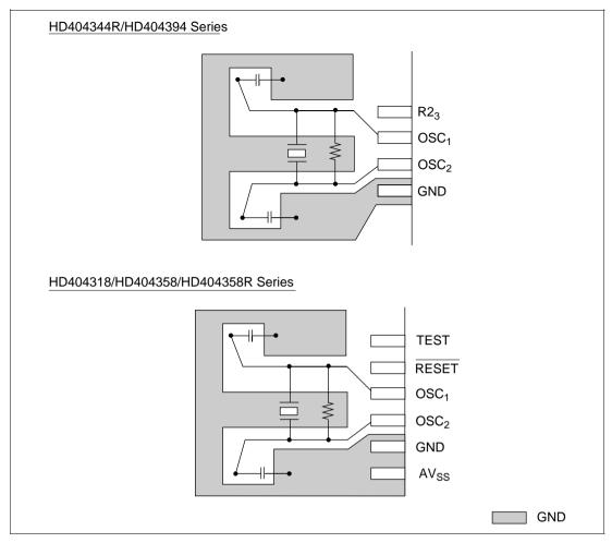
Figure 13-2 Wiring Examples for Crystal and Ceramic Oscillators
