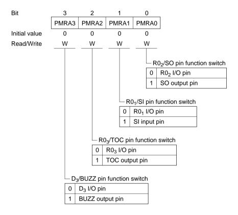
**Bit 2—R0<sub>3</sub>/TOC Pin Function Switch (PMRA2):** Selects whether the  $R0_3$ /TOC pin functions as the R0<sub>3</sub> I/O pin or as the timer C output pin (TOC).
