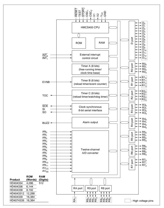
Figure 1-7 HD404339 Series Internal Block Diagram
