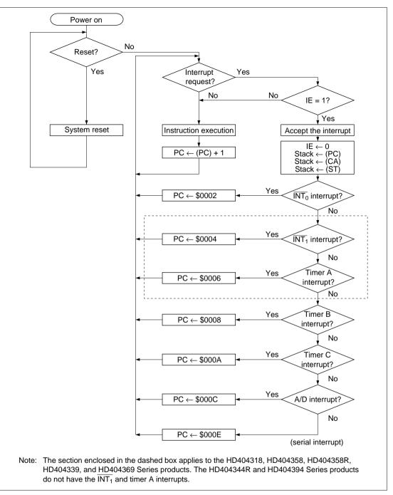
Figure 4-2 Interrupt Acceptance Flowchart
