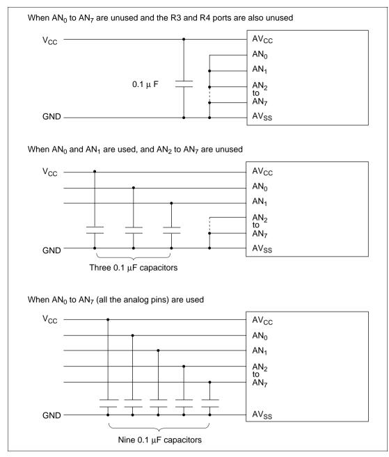
Figure 15-6 (a) Connection Examples for  $AV_{\rm CC}/AV_{\rm SS}$  and  $AV_{\rm SS}$  and the Used Analog Pins (HD404318 Series)
