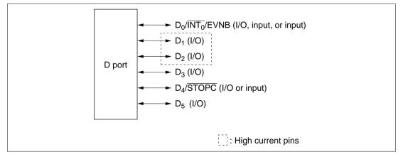
Figure 7-2 D Port Structure
