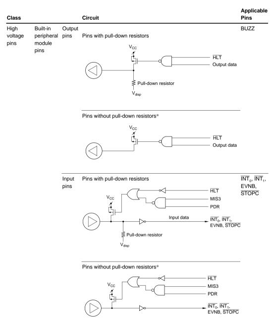
Note: \* The ZTAT<sup>™</sup> versions of these microcomputers only support pins without pull-down resistors.
