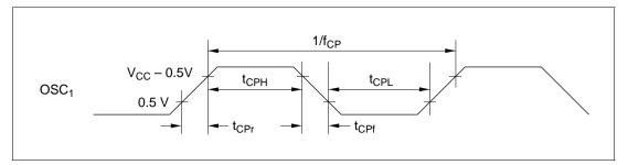
Figure 25-13 External Clock Timing (HD404318 Series)
