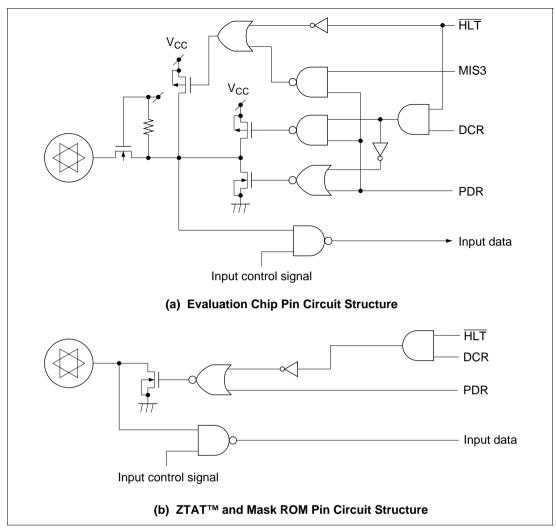
Figure 12-4 Medium Voltage NMOS Open Drain Pin Circuits
