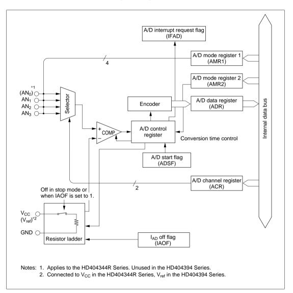
Figure 15-1 (a) A/D Converter Block Diagram (HD404344R/HD404394 Series)
