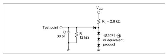
Figure 25-12 Timing Load Circuit
