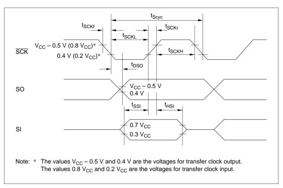
Figure 25-35 Serial Interface Timing (HD404369 Series)
