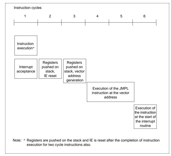
Figure 4-3 Interrupt Handling Sequence
