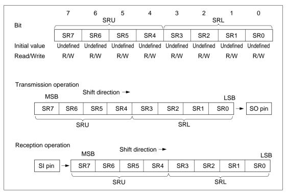
The SRL/U pair is undefined on reset and in stop mode.
