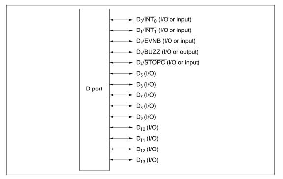
Figure 12-1 D Port Structure
