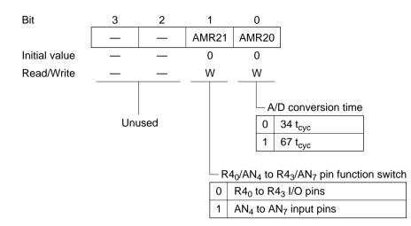
**Bit 1—R4<sub>0</sub>/AN<sub>4</sub> to R4<sub>3</sub>/AN<sub>7</sub> Pin Function Switch (AMR21):** Selects whether the R4<sub>0</sub>/AN<sub>4</sub> to R4<sub>3</sub>/AN<sub>7</sub> pins function as the R4<sub>0</sub> to R4<sub>3</sub> I/O pins or as the A/D converter channel 4 to 7 input pins (AN<sub>4</sub> to AN<sub>7</sub>).
