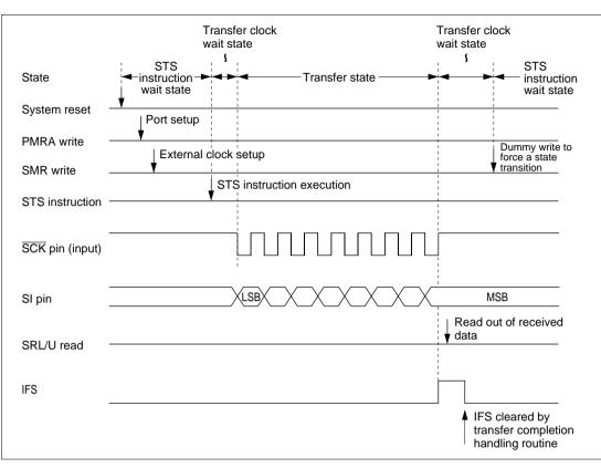
Figure 20-10 shows the operation sequence for data reception in external clock mode.
