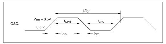
Figure 25-7 External Clock Timing (HD404394 Series)
