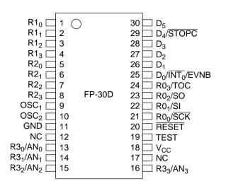
Note: No connections should be made to NC pins.
