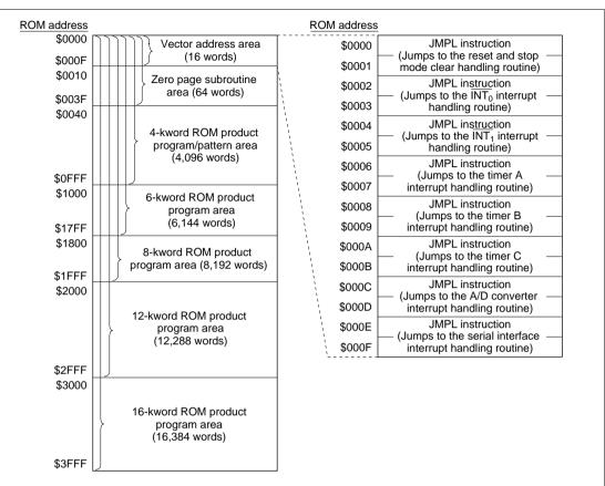
Figure 2-2 shows the memory map for the microcomputers in the HD404318, HD404358, HD404358R, HD404339, and HD404369 Series.
