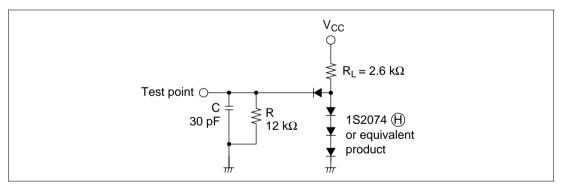
Figure 25-36 Timing Load Circuit
