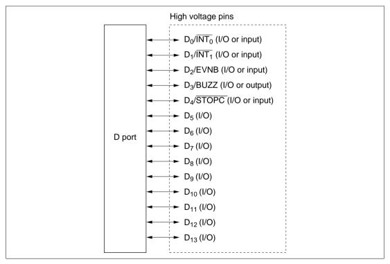
Figure 11-1 D Port Structure
