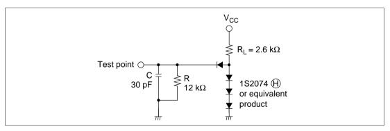
Figure 25-30 Timing Load Circuit
