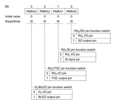
Bit 3— $D_3$ /BUZZ Pin Function Switch (PMRA3): Selects whether the  $D_3$ /BUZZ pin functions as the  $D_3$  input pin or as the alarm output pin (BUZZ).
