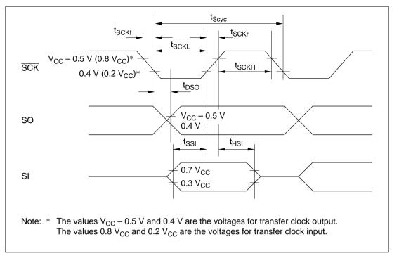
Figure 25-23 Serial Interface Timing (HD404358 and HD404358R Series)
