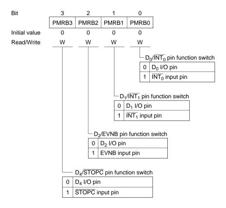
**Bit 3—D\_4/\overline{\text{STOPC}} Pin Function Switch (PMRB3):** Selects whether the  $D_4/\overline{\text{STOPC}}$  pin is used as the  $D_4$  I/O pin or as the STOPC input pin. The PMRB3 bit is cleared to 0 only on reset.
