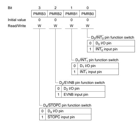
**Bit 3—D\_4/\overline{\text{STOPC}} Pin Function Switch (PMRB3):** Selects whether the  $D_4/\overline{\text{STOPC}}$  pin is used as the  $D_4$  I/O pin or as the stop mode clear pin (STOPC).
