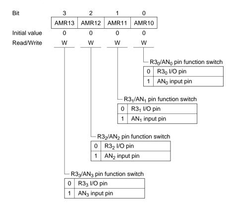
**Bit 3—R3<sub>3</sub>/AN<sub>3</sub> Pin Function Switch (AMR13):** Selects whether the  $R3_3/AN_3$  pin functions as the R3<sub>3</sub> I/O pin or as the A/D converter channel 3 input pin AN<sub>3</sub>.
