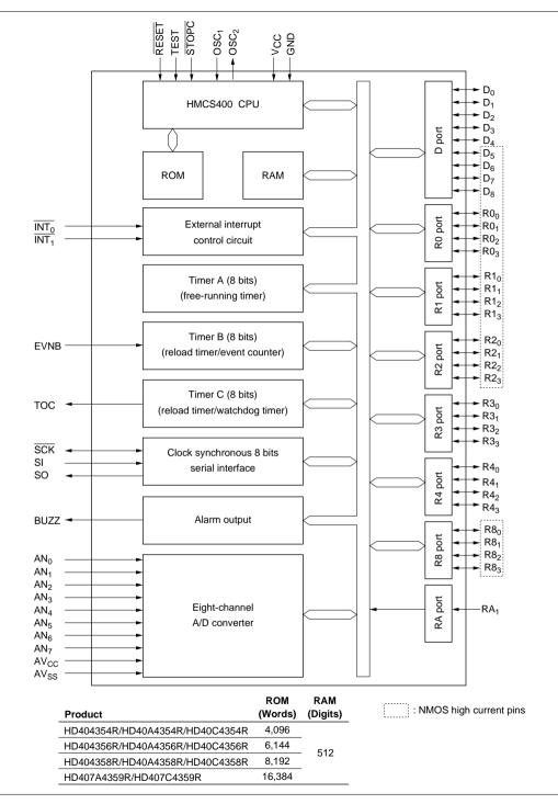
Figure 1-6 HD404358R Series Internal Block Diagram
