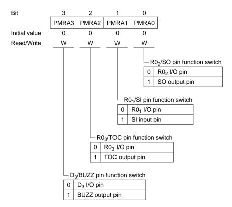
Bit 3— $D_3$ /BUZZ Pin Function Switch (PMRA3): Selects whether the  $D_3$ /BUZZ pin functions as the  $D_3$  I/O pin or as the alarm output pin (BUZZ).
