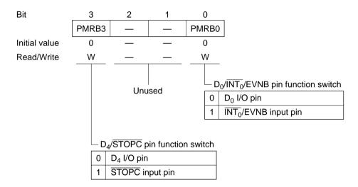
**Bit 0—D<sub>0</sub>/INT<sub>0</sub>/EVNB Pin Function Switch (PMRB0):** Selects whether the  $D_0/\overline{INT_0}$ /EVNB pin functions as the D0 I/O pin or as the external interrupt 0/timer B event ( $\overline{INT_0}$ /EVNB) input pin.
