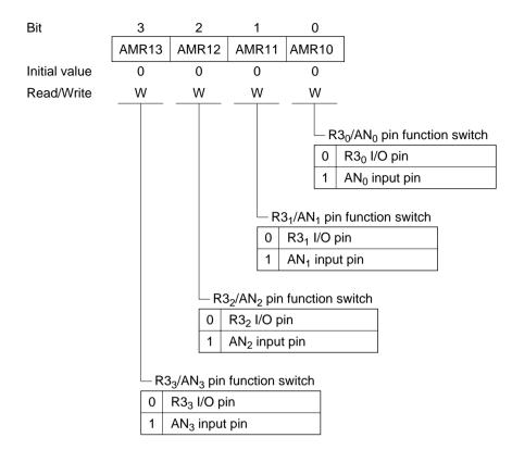
**Bit 3—R3<sub>3</sub>/AN<sub>3</sub> Pin Function Switch (AMR13):** Selects whether the  $R3_3/AN_3$  pin functions as the R3<sub>3</sub> I/O pin or as the A/D converter channel 3 input pin AN<sub>3</sub>.
