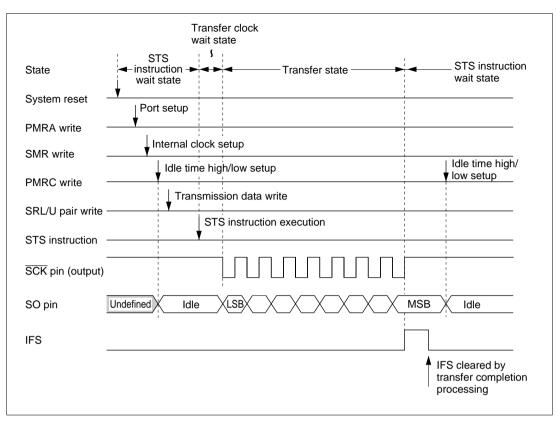
Figure 20-8 Serial Transmission Operation Sequence (Internal Clock Mode)
