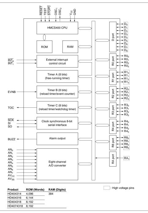
Figure 1-4 HD404318 Series Internal Block Diagram
