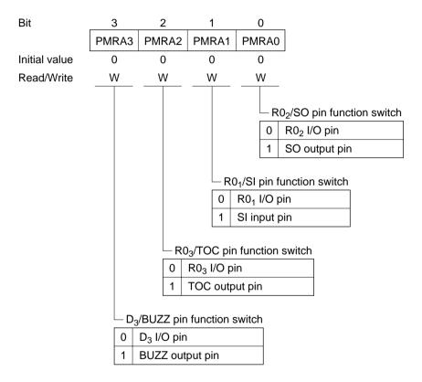
Bit 3—D<sub>3</sub>/BUZZ Pin Function Switch (PMRA3): Selects whether the  $D_3$ /BUZZ pin functions as the  $D_3$  I/O pin or as the alarm output pin (BUZZ).
