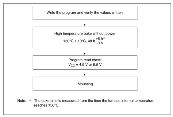
Figure 22-11 Recommended Screening Procedure
