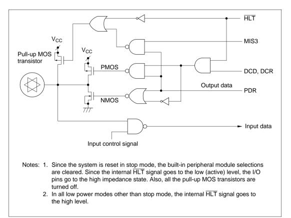
Figure 7-1 I/O Pin Circuit Structure
