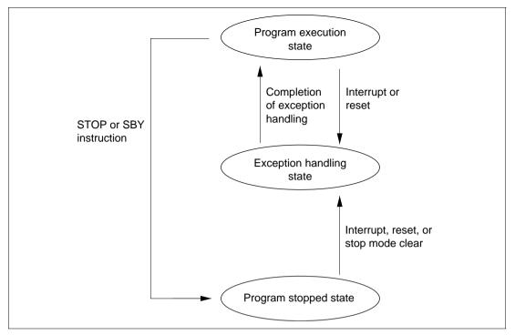
Figure 3-6 State Transition Diagram
