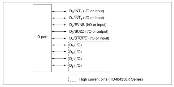
Figure 10-1 D Port Structure
