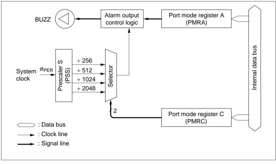
Figure 21-1 Alarm Output Circuit Block Diagram
