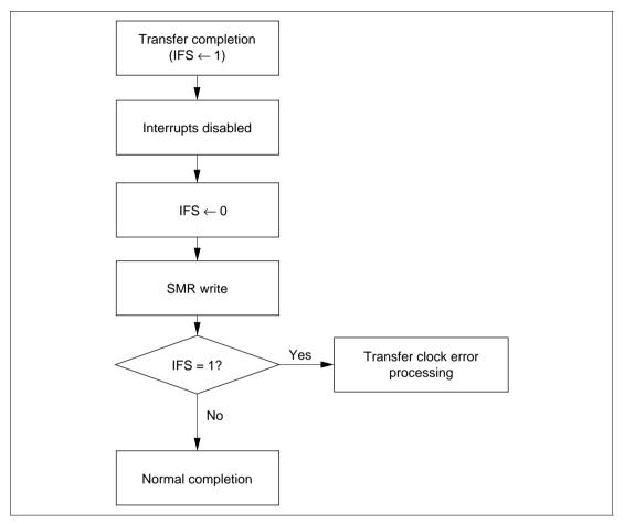
Figure 20-16 Transfer Clock Error Detection Flowchart
