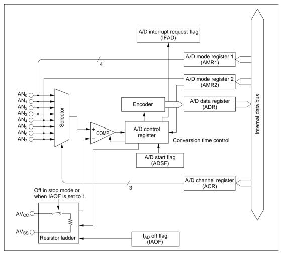
Figure 15-1 (b) A/D Converter Block Diagram (HD404318/HD404358/HD404358R Series)
