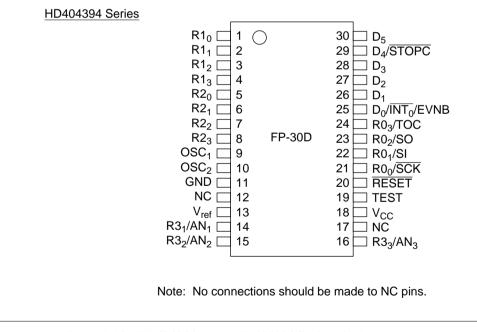
Figure 1-10 HD404344R and HD404394 Series Pin Arrangements (FP-30D Package: Top View)
