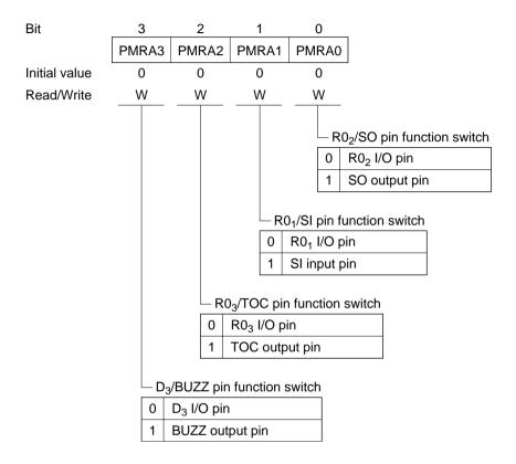
**Bit 2—R0<sub>3</sub>/TOC Pin Function Switch (PMRA2):** Selects whether the R0<sub>3</sub>/TOC pin functions as the R0<sub>3</sub> I/O pin or as the timer C output pin (TOC).
