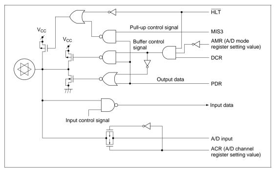
Figure 15-5 R Port/Analog Input Shared Function Pin Circuit
