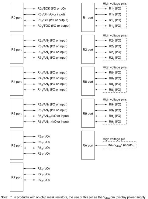
In products with on-chip mask resistors, the use of this pin as the V<sub>disp</sub> pin (display power supply pin) can be selected as a mask option.
