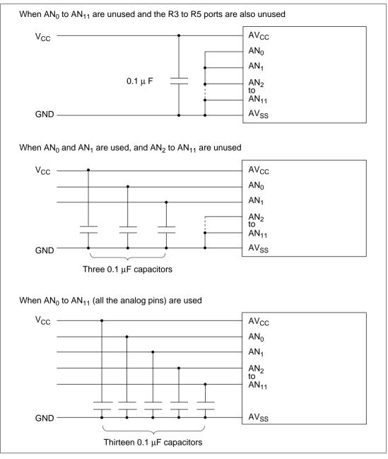
Figure 15-6 (b) Connection Examples for  $AV_{\rm CC}/AV_{\rm SS}$  and  $AV_{\rm SS}$  and the Used Analog Pins (HD404339 Series)
