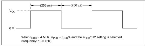
Figure 21-2 Alarm Output Waveform Example
