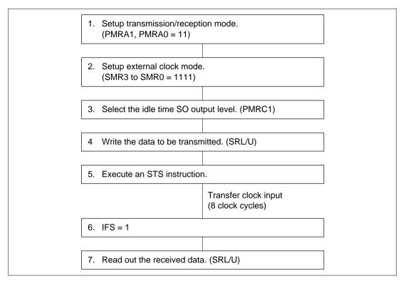
Figure 20-13 Simultaneous Transmission and Reception Procedure (External Clock Mode)
