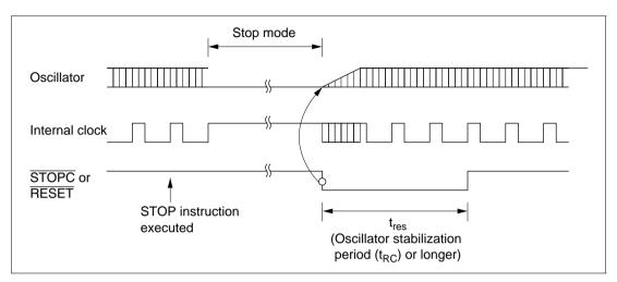
Figure 6-4 Stop Mode Clear Timing
