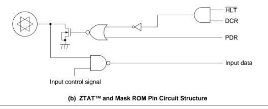
Figure 8-4 Medium Voltage NMOS Open Drain Pin Circuits
