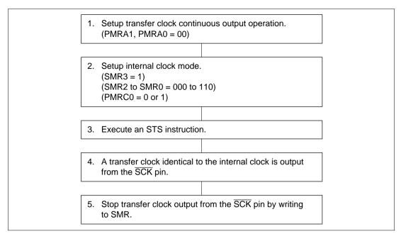
Figure 20-15 Transfer Clock Continuous Output Operation Procedure
