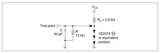
Figure 25-6 Timing Load Circuit
