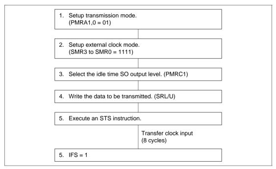
Figure 20-5 Data Transmission Procedure (External Clock Mode)
