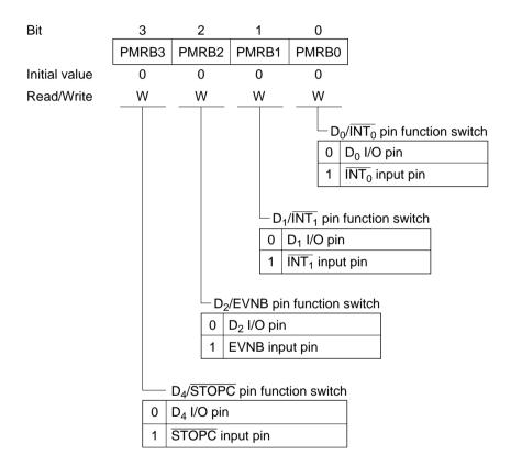
**Bit 3—D\_4/\overline{\text{STOPC}} Pin Function Switch (PMRB3):** Selects whether the  $D_4/\overline{\text{STOPC}}$  pin is used as the  $D_4$  I/O pin or as the STOPC input pin.
