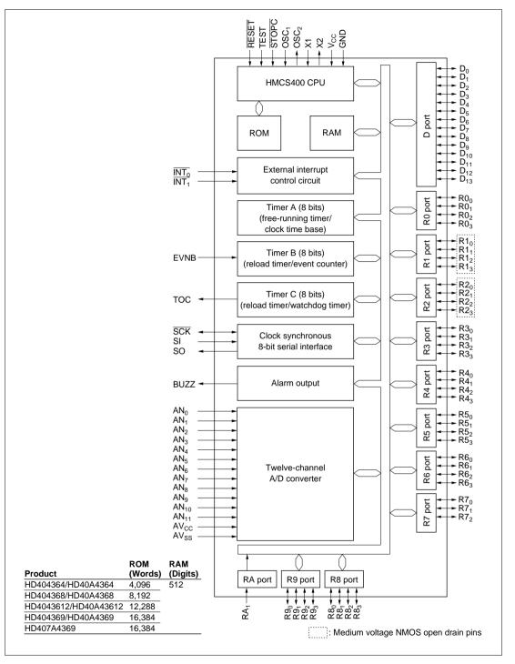
Figure 1-8 HD404369 Series Internal Block Diagram
