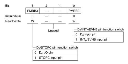
**Bit 3—D\_4/\overline{\text{STOPC}} Pin Function Switch (PMRB3):** Selects whether the  $D_4/\overline{\text{STOPC}}$  pin is used as the  $D_4$  I/O pin or as the STOPC input pin.
