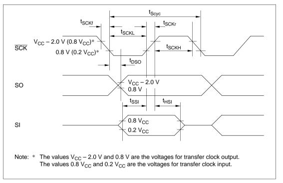
Figure 25-17 Serial Interface Timing (HD404318 Series)
