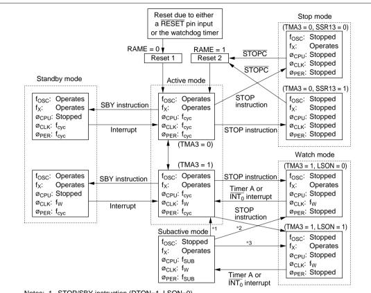
Figure 6-1 shows the state transition diagram for the low power modes.
