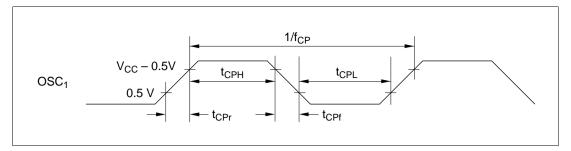
Figure 25-31 External Clock Timing (HD404369 Series)
