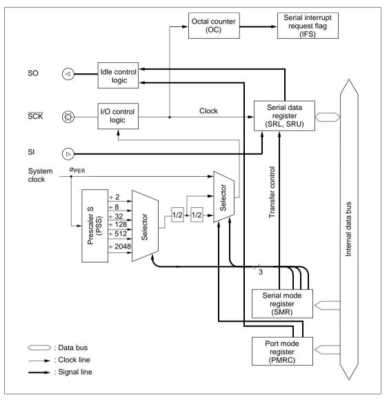
Figure 20-1 Serial Interface Block Diagram
