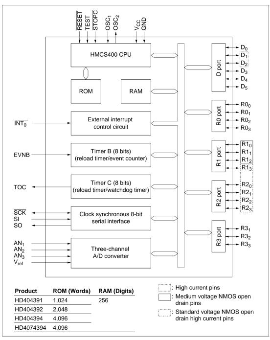
Figure 1-3 HD404394 Series Internal Block Diagram
