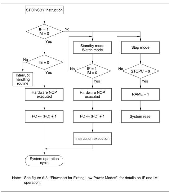
Figure 6-7 Low Power Mode Operating Sequence
