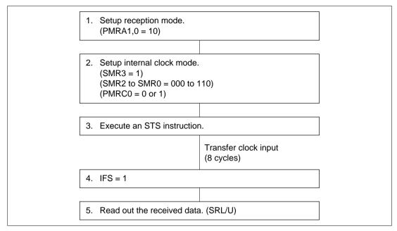
Figure 20-11 Data Reception Procedure (Internal Clock Mode)
