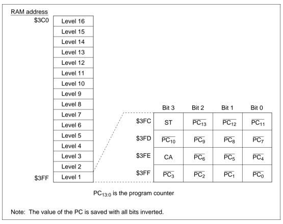
Figure 2-17 Stack Area Structure
