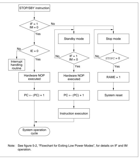
Figure 5-4 Low Power Mode Operating Sequence
