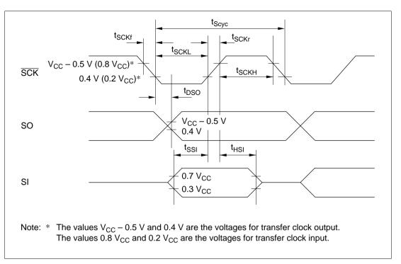
Figure 25-11 Serial Interface Timing
