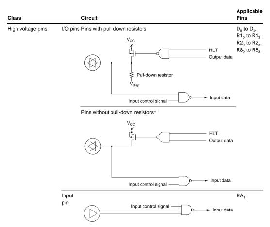
Note: \* The ZTAT<sup>™</sup> versions of these microcomputers only support pins without pull-down resistors.
