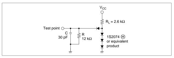
Figure 25-24 Timing Load Circuit
