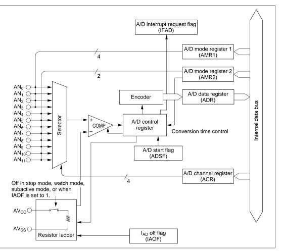
Figure 15-1 (c) A/D Converter Block Diagram (HD404339/HD404369 Series)
