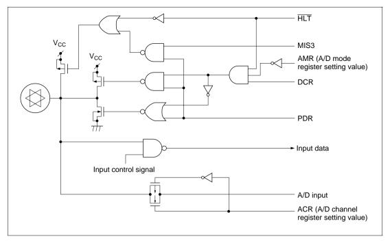
Figure 12-3 R Port/Analog Input Shared Function Pin Circuit
