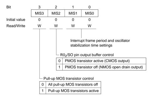
**Bit 3—Pull-Up MOS Transistor Control (MIS3):** Controls the on/off states of the pull-up MOS transistors built into the I/O port pins.
