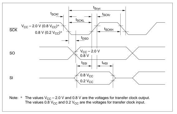
Figure 25-29 Serial Interface Timing (HD404339 Series)
