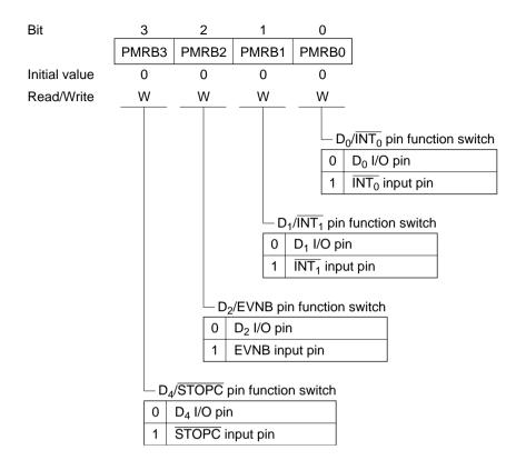
**Bit 3—D**<sub>4</sub>/STOPC Pin Function Switch (PMRB3): Selects whether the D<sub>4</sub>/STOPC pin is used as the D<sub>4</sub> I/O pin or as the stop mode clear pin (STOPC).
