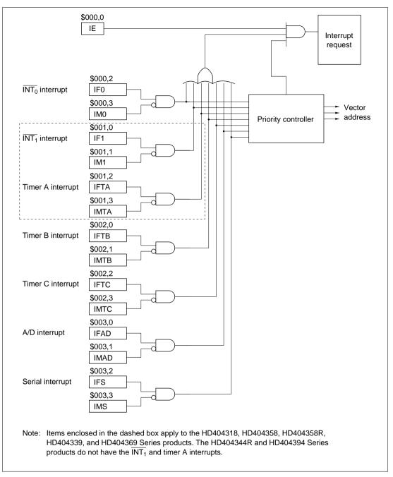
Figure 4-1 Interrupt Controller Block Diagram
