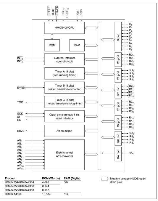
Figure 1-5 HD404358 Series Internal Block Diagram
