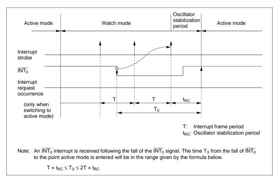
Figure 6-5 Watch Mode to Active Mode Transition Timing
