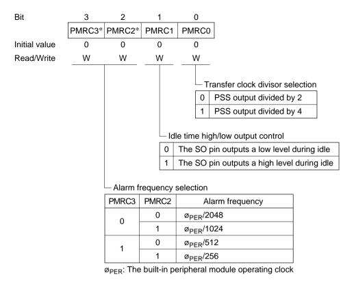
Note: \* Applies to the HD404318, HD404358, HD404358R, HD404339, and HD404369 Series. The PMRC3 and PMRC2 bits are unused in the HD404344R and HD404394 Series.
