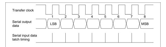
Figure 20-3 Clock Synchronous Serial Data Transfer Format
