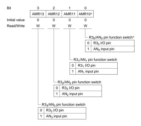
Note: \* Applies to the HD404344R, HD404318, HD404358, HD404358R, HD404339, and HD404369 Series. The AMR10 bit is unused in the HD404394 Series.
