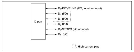
Figure 8-1 D Port Structure
