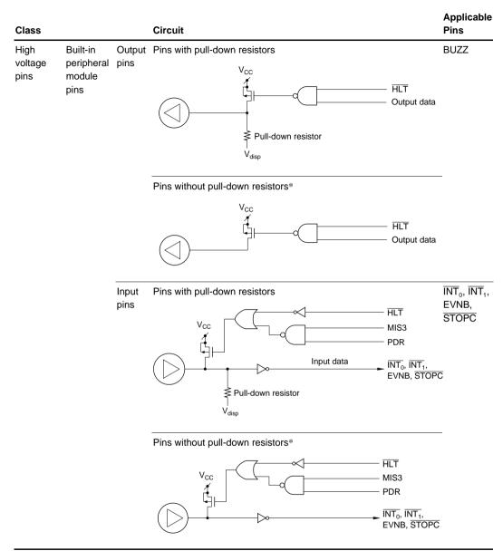
Note: \* The ZTAT<sup>™</sup> versions of these microcomputers only support pins without pull-down resistors.
