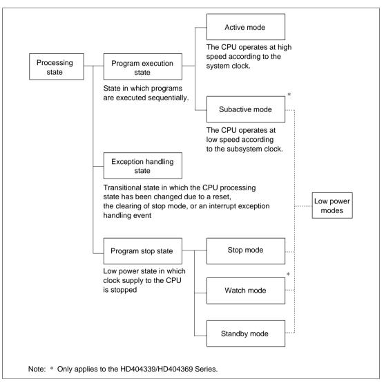
Figure 3-5 Processing State Classification
