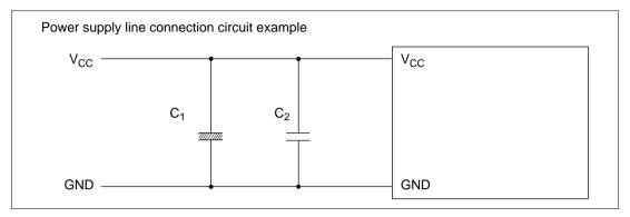
Figure 15-7  $V_{\rm CC}$  to Ground Circuit Example
