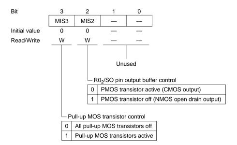
**Bit 3—Pull-Up MOS Transistor Control (MIS3):** Controls the on/off states of the pull-up MOS transistors built into the I/O port pins.
