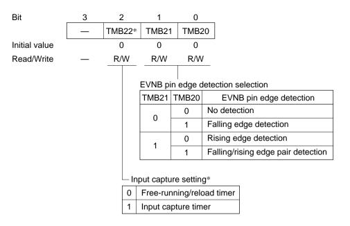
Note: \* Applies to the HD404318, HD404358, HD404358R, HD404339, and HD404369 Series. The TMB22 bit is unused in the HD404344R and HD404394 Series.
