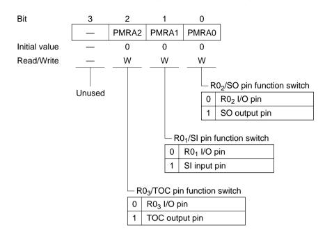
**Bit 2—R0<sub>3</sub>/TOC Pin Function Switch (PMRA2):** Selects whether the R0<sub>3</sub>/TOC pin functions as the R0<sub>3</sub> input pin or as the timer C output pin (TOC).
