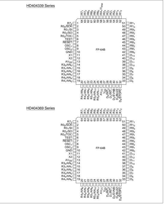
Figure 1-14 HD404339 and HD404369 Series Pin Arrangements (FP-64B Package: Top View)
