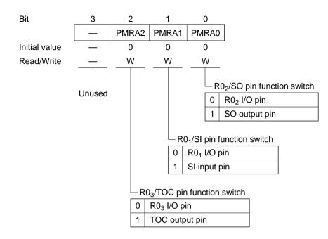
**Bit 2—R0<sub>3</sub>/TOC Pin Function Switch (PMRA2):** Selects whether the  $R0_3$ /TOC pin functions as the R0<sub>3</sub> I/O pin or as the timer C output pin (TOC).
