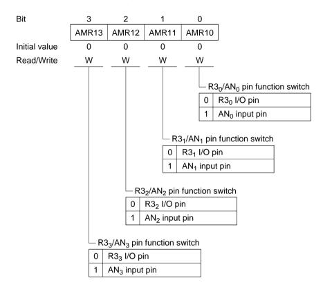
**Bit 3—R3<sub>3</sub>/AN<sub>3</sub> Pin Function Switch (AMR13):** Selects whether the R3<sub>3</sub>/AN<sub>3</sub> pin functions as the R3<sub>3</sub> I/O pin or as the A/D converter channel 3 input pin AN<sub>3</sub>.
