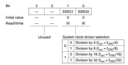
**Bits 1 and 0—System Clock Selection (SSR21, SSR20):** These bits set the system clock divisor to be 4, 8, 16, or 32, i.e., the system oscillator frequency is divided by 4, 8, 16, or 32. ( $f_{cyc} = f_{OSC}/4$ ,  $f_{OSC}/8$ ,  $f_{OSC}/16$ , or  $f_{OSC}/32$ ) This setting only takes effect when watch mode is entered. That is, the system clock must be stopped to change the divisor.
