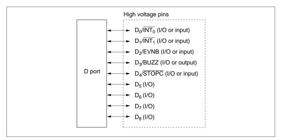
Figure 9-1 D Port Structure
