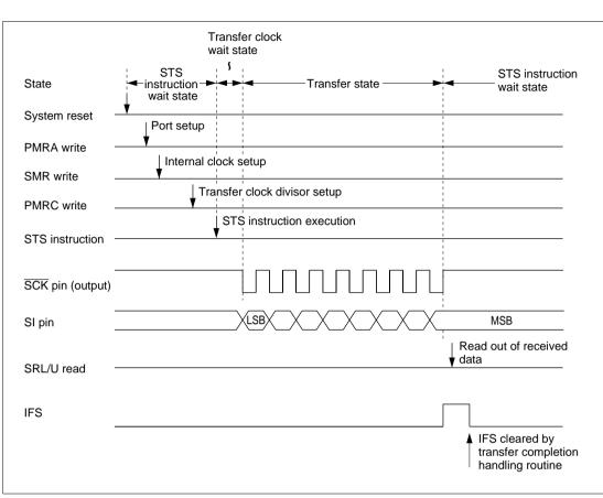
Figure 20-12 shows the operation sequence for data reception in internal clock mode.
