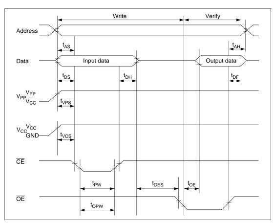
Figure 22-10 shows the PROM write/verify timing.
