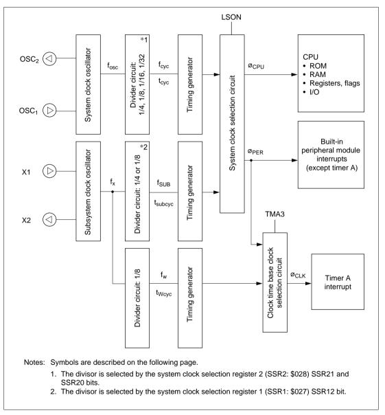
Figure 14-1 shows the block diagram of the oscillator circuits used in the HD404339 and HD404369 Series microcomputers.
