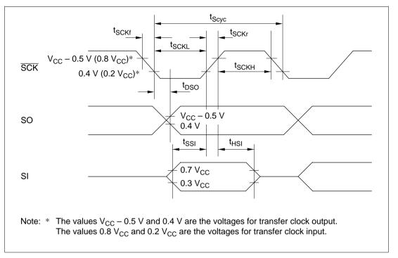
Figure 25-5 Serial Interface Timing
