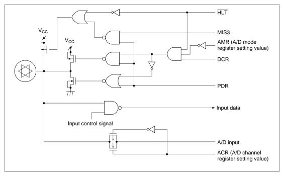
Figure 10-3 R Port/Analog Input Shared Function Pin Circuit
