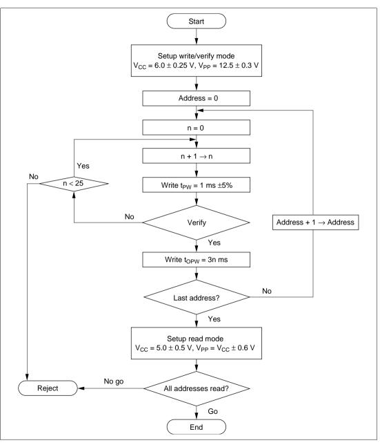
Figure 22-9 Flowchart for High-Speed Programming
