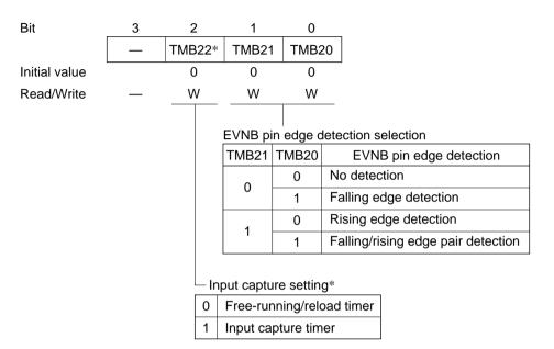
Note: \* Applies to the HD404318, HD404358, HD404358R, HD404339, and HD404369 Series. TMB22 is unused in the HD404344R and HD404394 Series.
