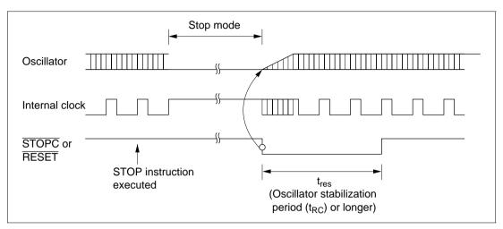
Figure 5-3 Stop Mode Clear Timing
