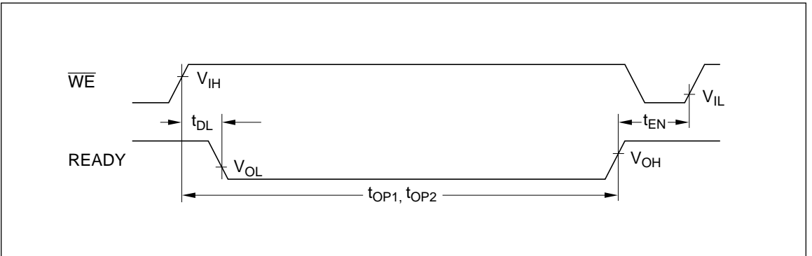
Figure 29 READY Timing (When the READY Output Is Always Available)
