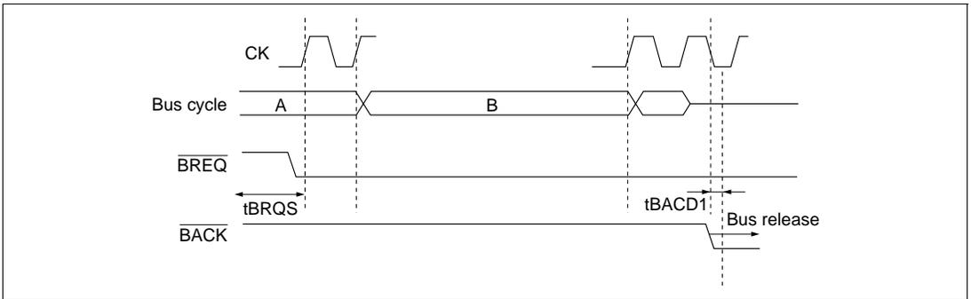
**Figure 8.43** When  $\overline{\text{BREQ}}$  is Input without Satisfying  $t_{\text{BRQS}}$
