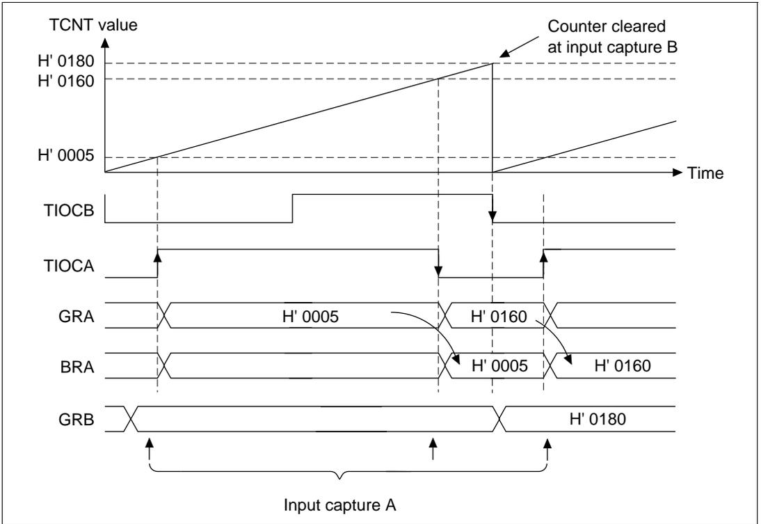
**Figure 10.50 Buffer Mode Operation Example 2 (Input Capture Register)**
