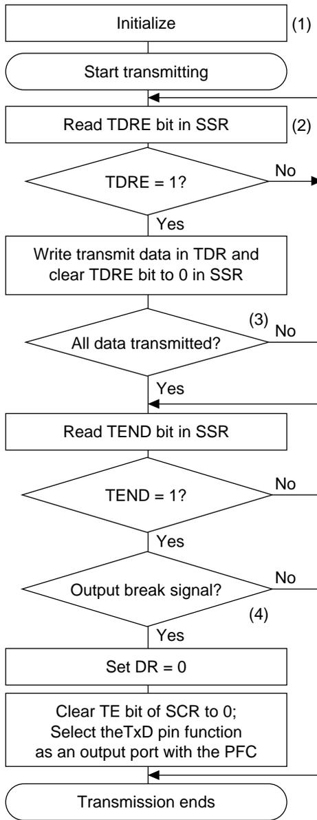
**Figure 13.5 Sample Flowchart for Transmitting Serial Data**
