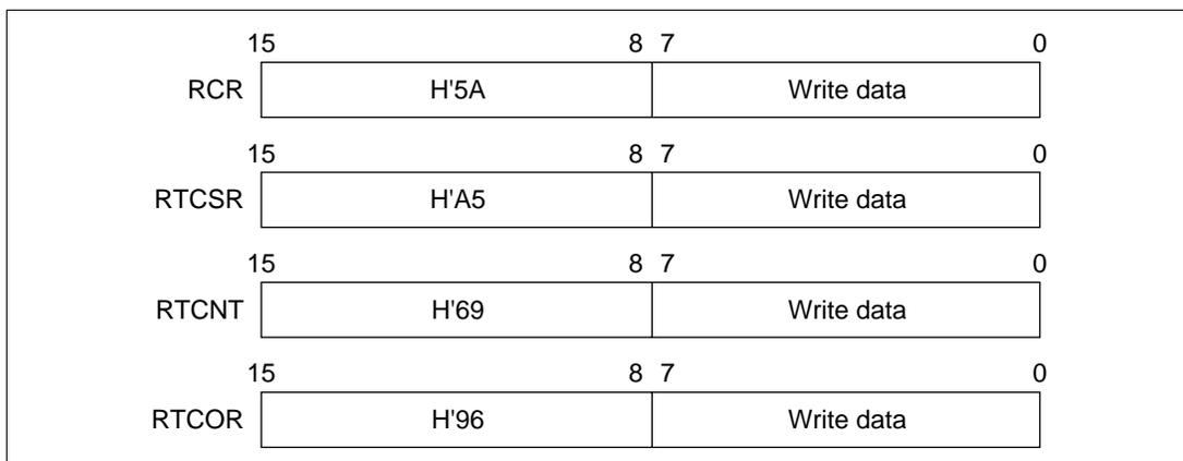
**Figure 8.2 Writing to RCR, RTCSR, RTCNT, and RTCOR**
