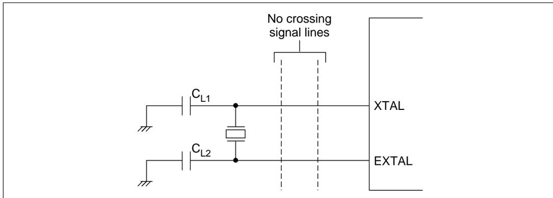
**Figure 7.6 Precaution on Oscillator Circuit Board Design**
