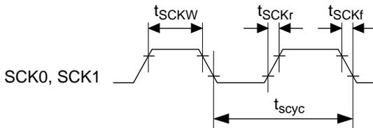
**Figure 20.71 Input Clock Timing**
