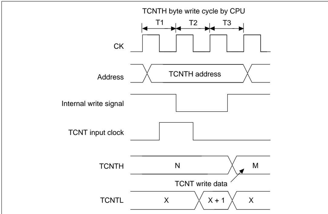
**Figure 10.60 Contention between TCNT Byte Write and Increment**
