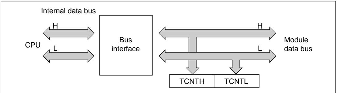
Figure 10.6 TCNT Access (CPU to TCNT (Word))
