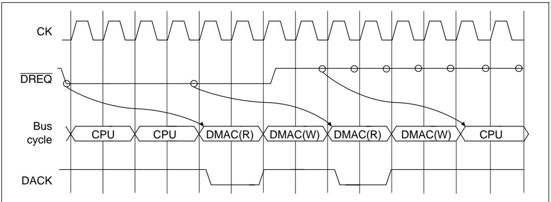
**Figure 9.24  $\overline{\text{DREQ}}$  Pin Sampling Timing in Burst Mode (Dual Address  $\overline{\text{DREQ}}$  Level Detection,  $\overline{\text{DACK}}$  Active-Low,  $\overline{\text{DACK}}$  Output in Read Cycle, 1 Bus Cycle = 2 States)**
