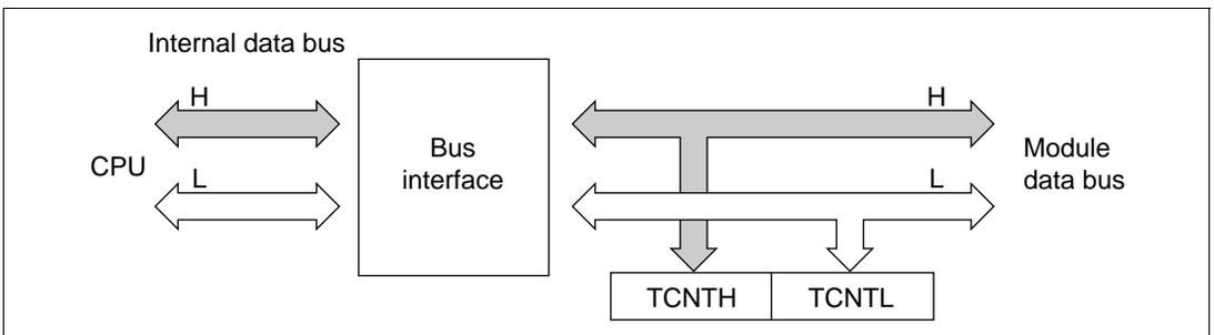
Figure 10.8 TCNT Access (CPU to TCNT (Upper Byte))
