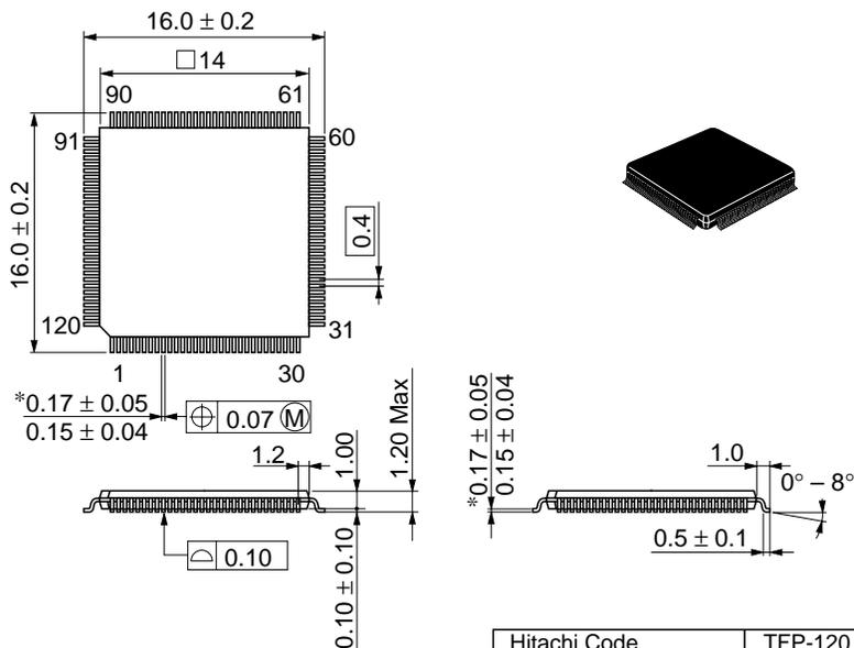
\*Dimension including the plating thickness
