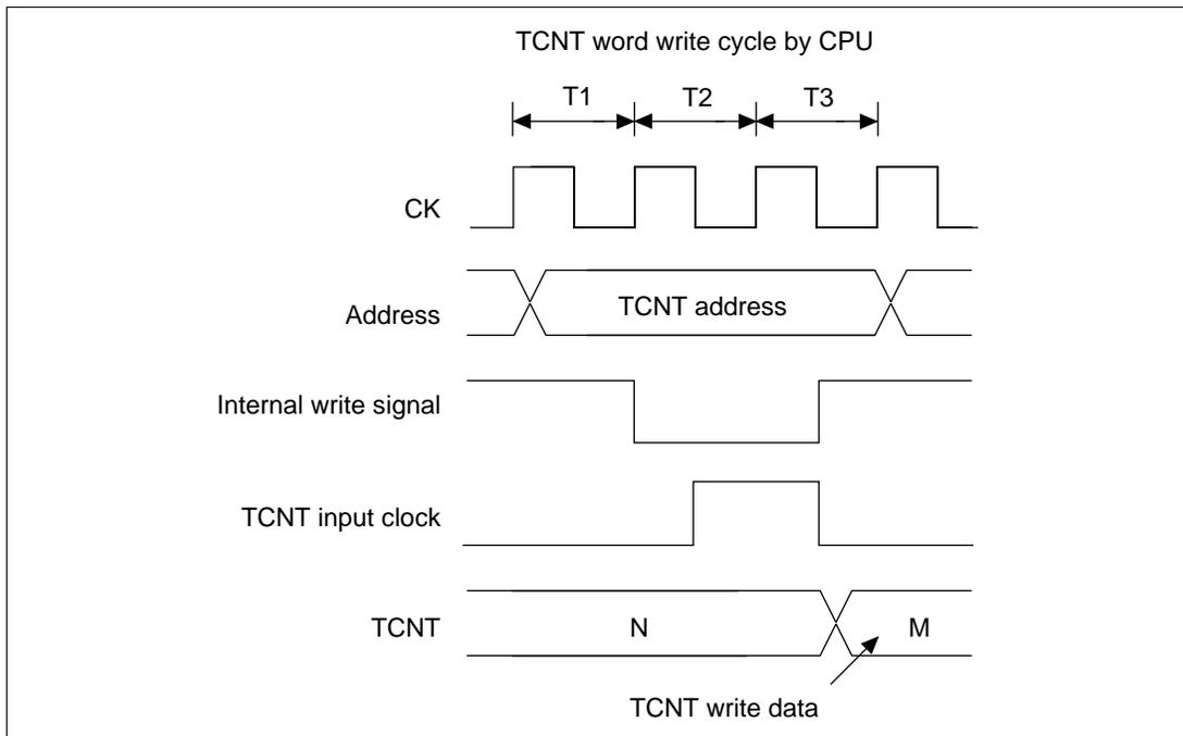
**Figure 10.59** Contention between TCNT Word Write and Increment
