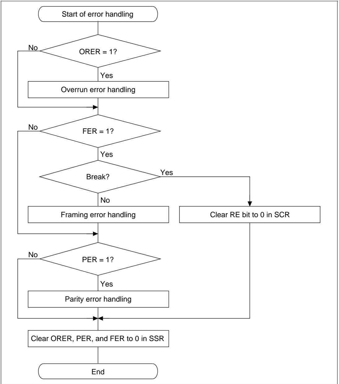
**Figure 13.7 Sample Flowchart for Receiving Serial Data (cont)**
