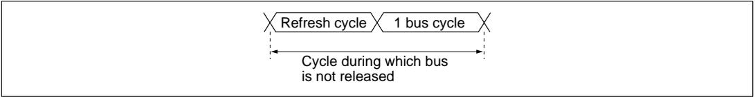
**Figure 8.46 Refresh Cycle and Following Bus Cycle**
