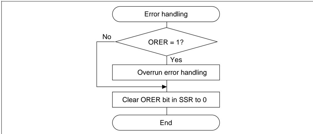
**Figure 13.18 Sample Flowchart for Serial Receiving (cont)**
