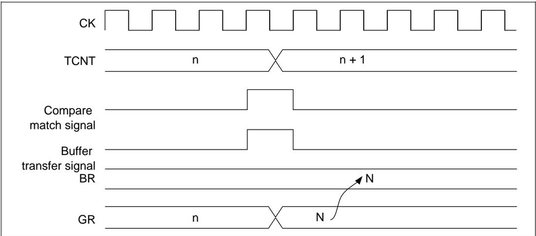
**Figure 10.49 Compare Match Timing Example for Buffer Operation**
