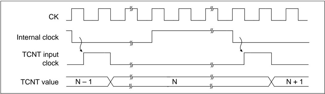
**Figure 10.17 Count Timing for Internal Clock Sources**
