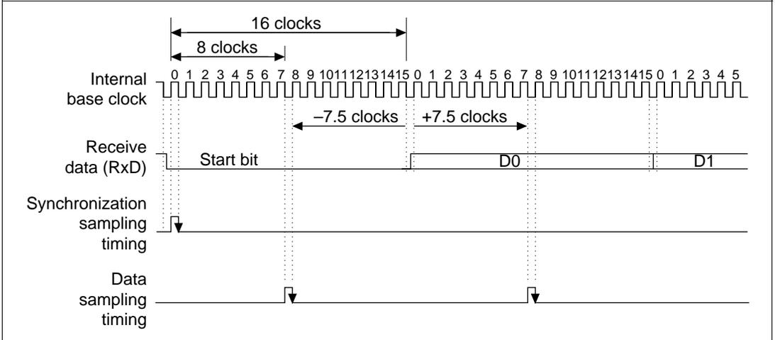
**Figure 13.21 Receive Data Sampling Timing in Asynchronous Mode**
