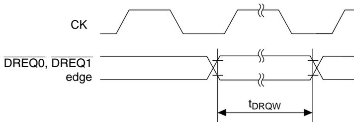
**Figure 20.35  $\overline{\text{DREQ0}}$ ,  $\overline{\text{DREQ1}}$  Input Timing (2)**
