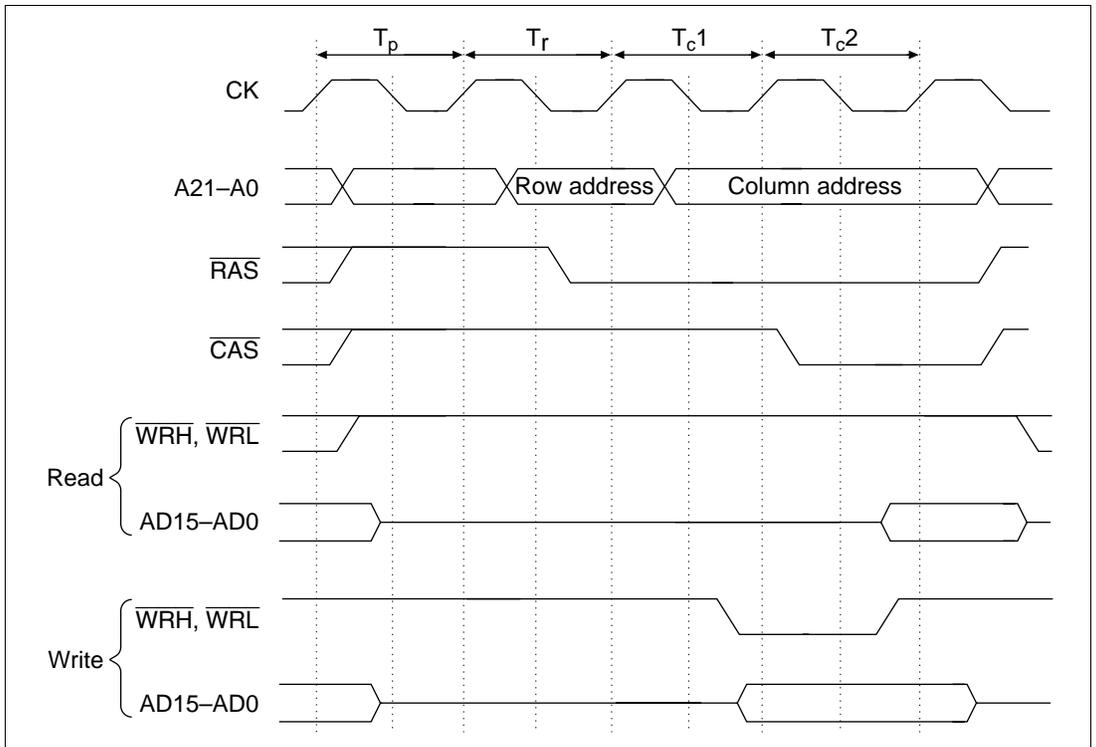
**Figure 8.18 Long Pitch Access Timing**
