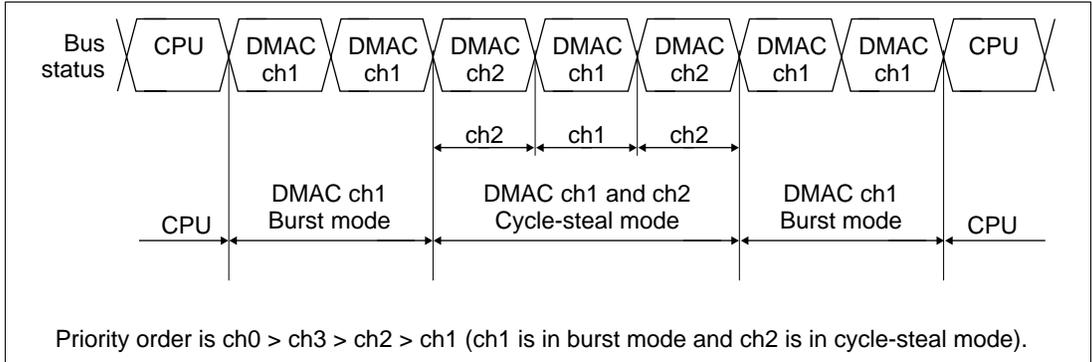
**Figure 9.12 Bus Handling when Multiple Channels are Operating**
