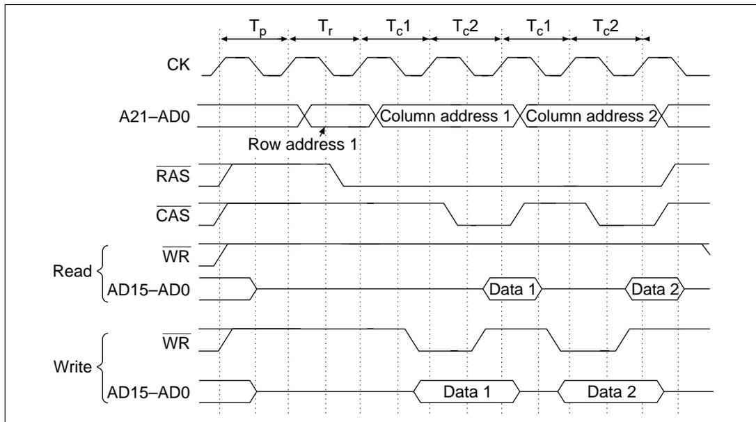
**Figure 8.26 Long-Pitch, High-Speed Page Mode (Read/Write Cycle)**
