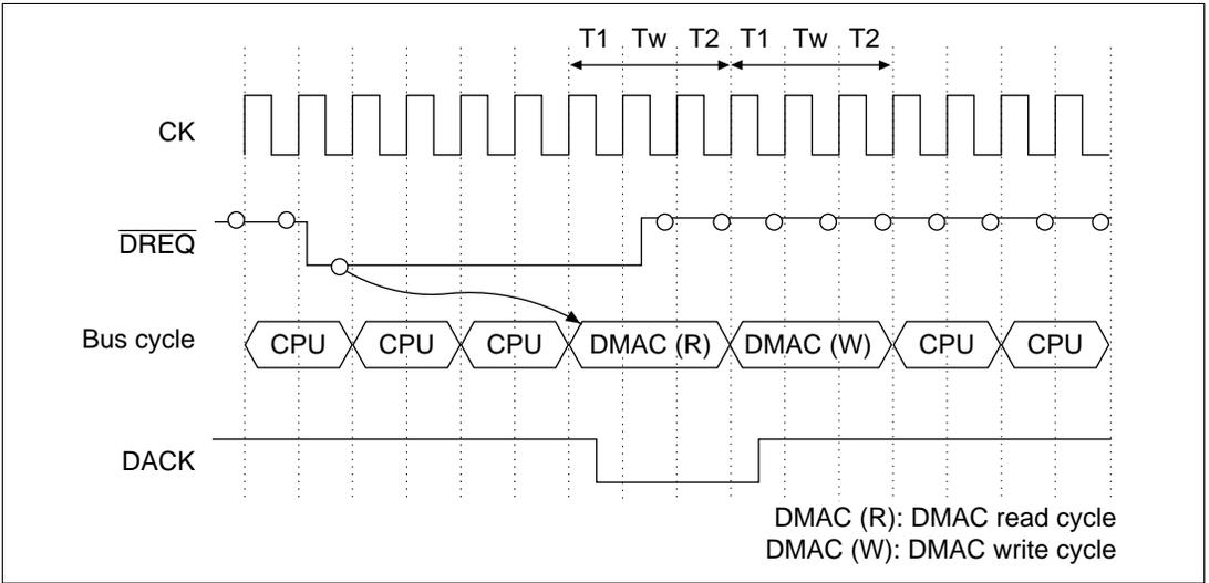
**Figure 9.18  $\overline{\text{DREQ}}$  Sampling Timing in Cycle-Steal Mode (Output with  $\overline{\text{DREQ}}$  Level Detection and DACK Active-Low) (Dual Address Mode, Bus Cycle = 2 States + 1 Wait State)**
