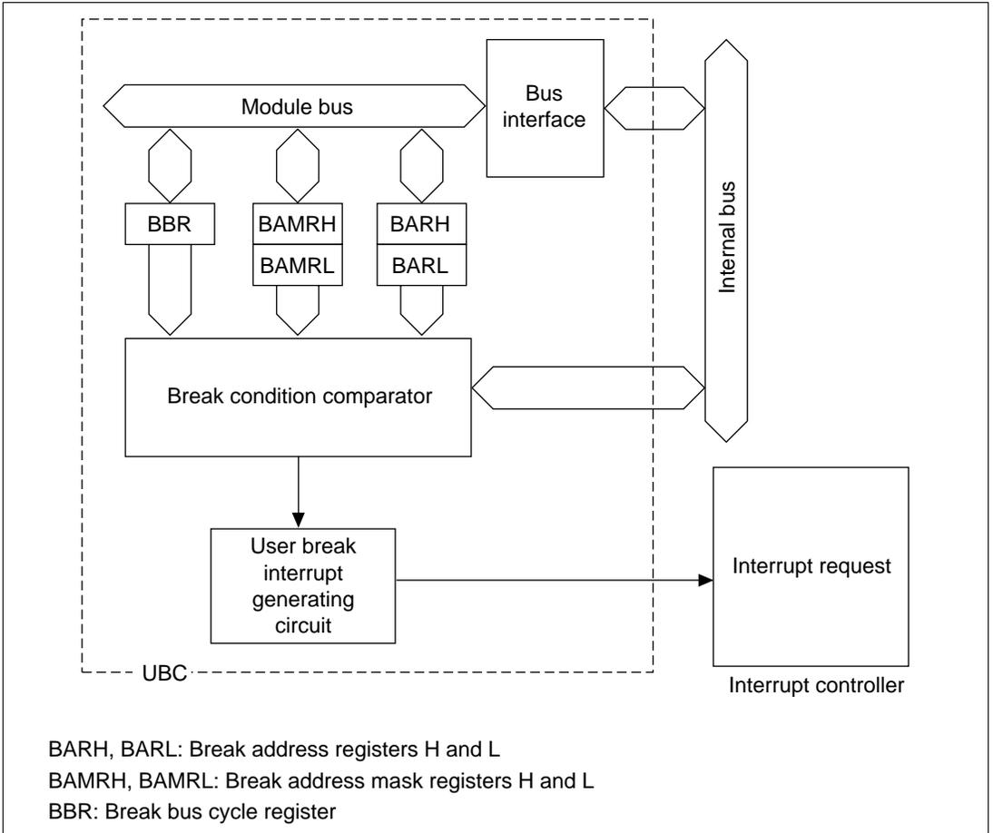
**Figure 6.1 Block Diagram of User Break Controller**
