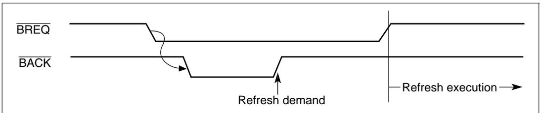
**Figure 8.36**  $\overline{\text{BACK}}$  Operation in Response to Refresh Demand (1)
