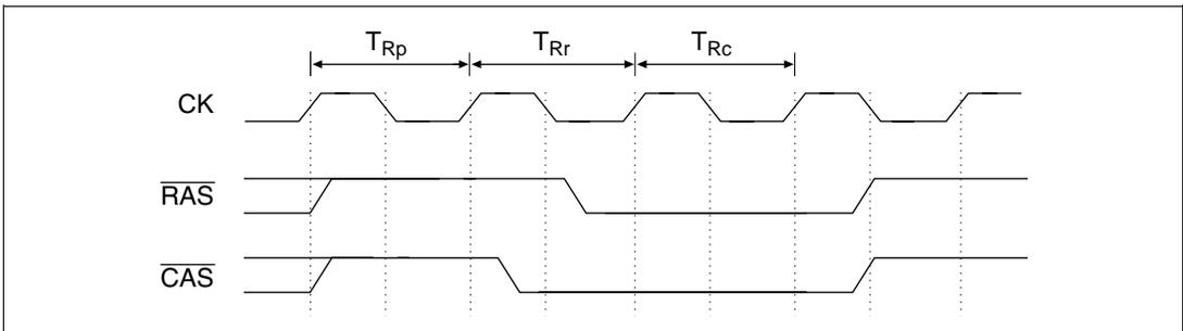
**Figure 8.30 Output Timing for CAS-Before-RAS Refresh Signal**
