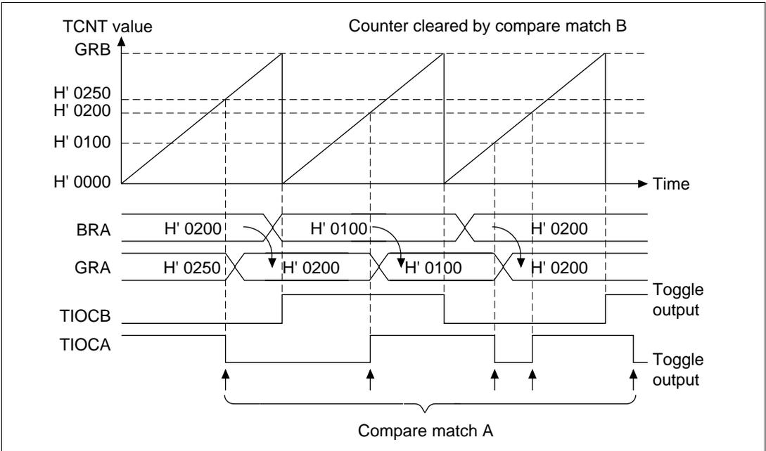
**Figure 10.48 Buffer Mode Operation Example 1 (Output Compare Register)**
