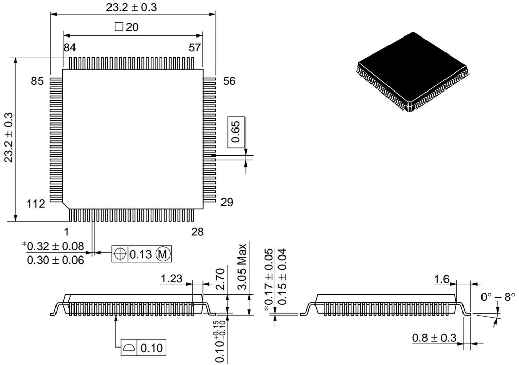
\*Dimension including the plating thickness
