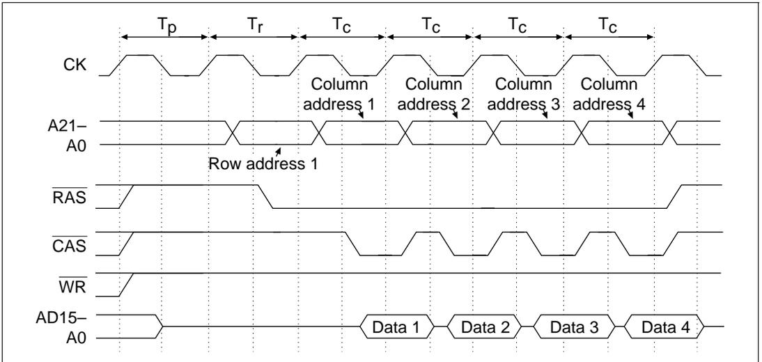
**Figure 8.23 Short-Pitch, High-Speed Page Mode (Read Cycle)**
