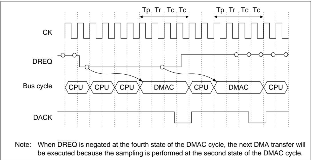
**Figure 9.19  $\overline{\text{DREQ}}$  Sampling Timing in Cycle-Steal Mode (Output with  $\overline{\text{DREQ}}$  Level Detection and DACK Active-Low) (Single Address Mode, Bus Cycle = DRAM Bus Cycle (Long Pitch Normal Mode))**
