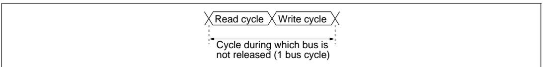
**Figure 8.45** TAS Instruction Read Cycle and Write Cycle
