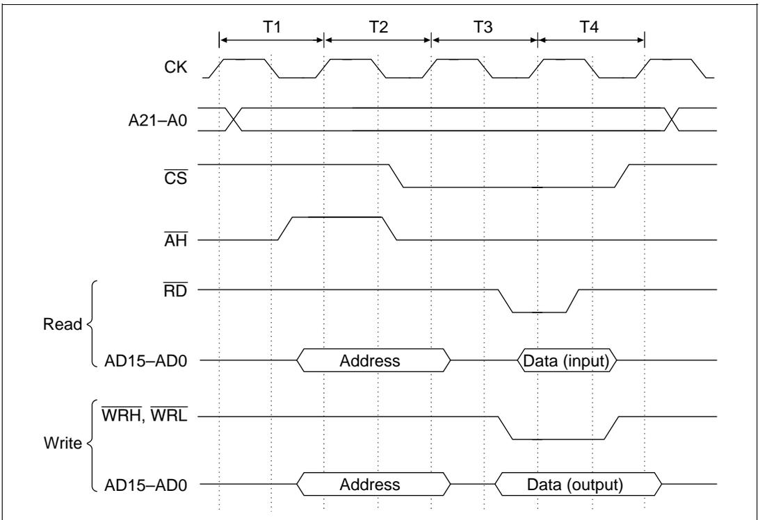
Figure 8.32 Access Timing For Address/Data Multiplexed I/O Space
