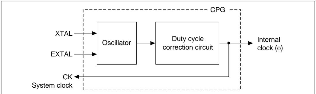
Figure 7.1 Block Diagram of Clock Pulse Generator
