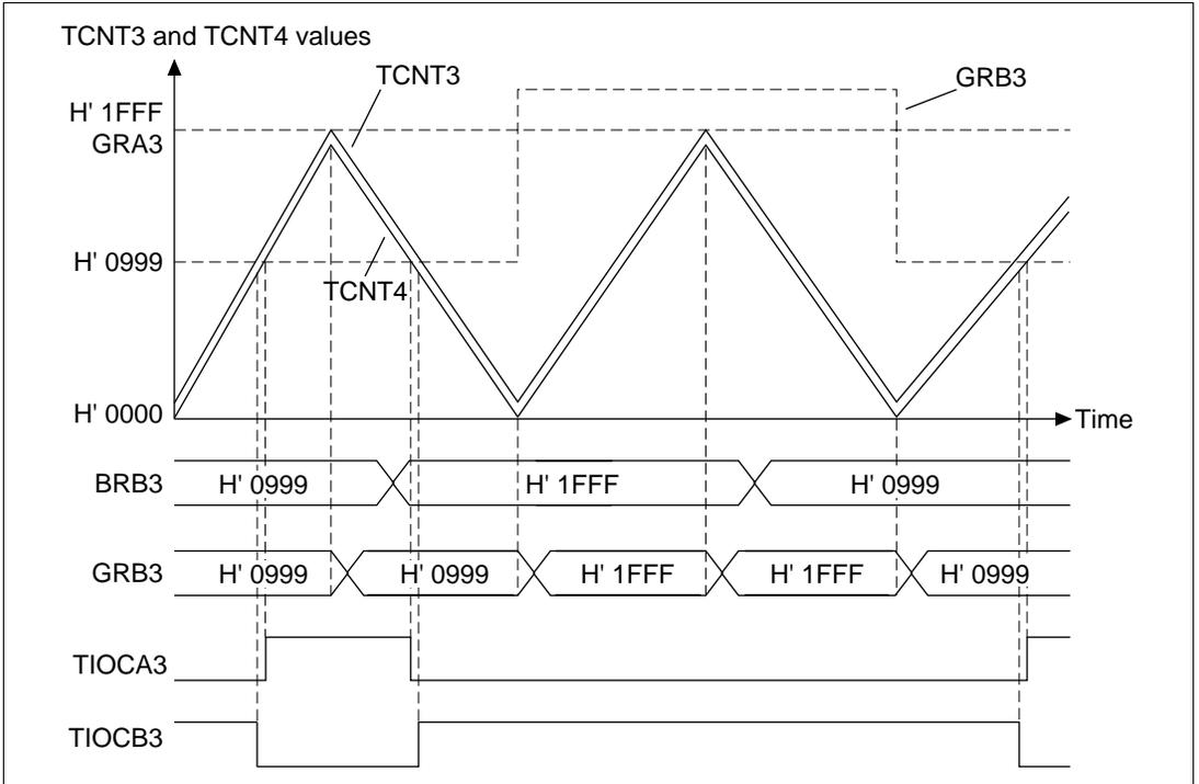
**Figure 10.52 Buffer Mode Operation Example 3 (Complementary PWM Mode)**
