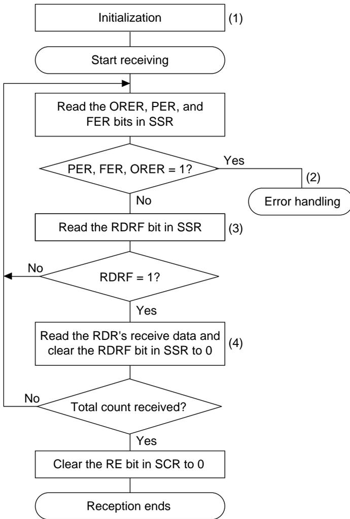
**Figure 13.7 Sample Flowchart for Receiving Serial Data**
