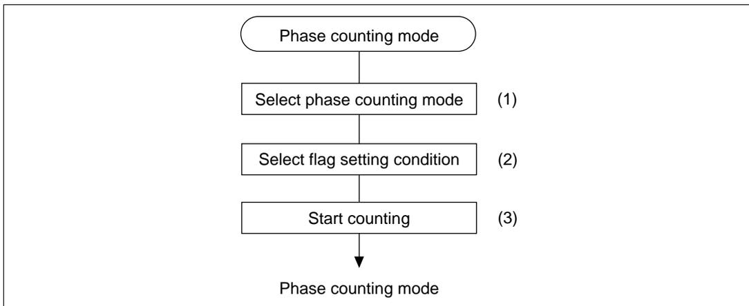
**Figure 10.42 Procedure for Selecting Phase Counting Mode**
