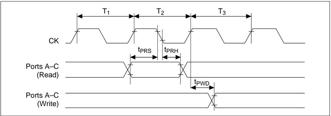
**Figure 20.38 Programmable Timing Pattern Controller Output Timing**
