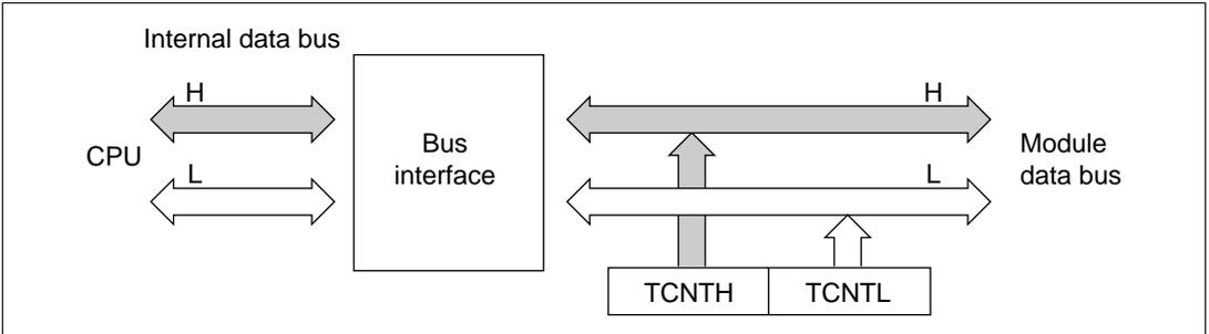
**Figure 10.10 TCNT Access (TCNT to CPU (Upper Byte))**
