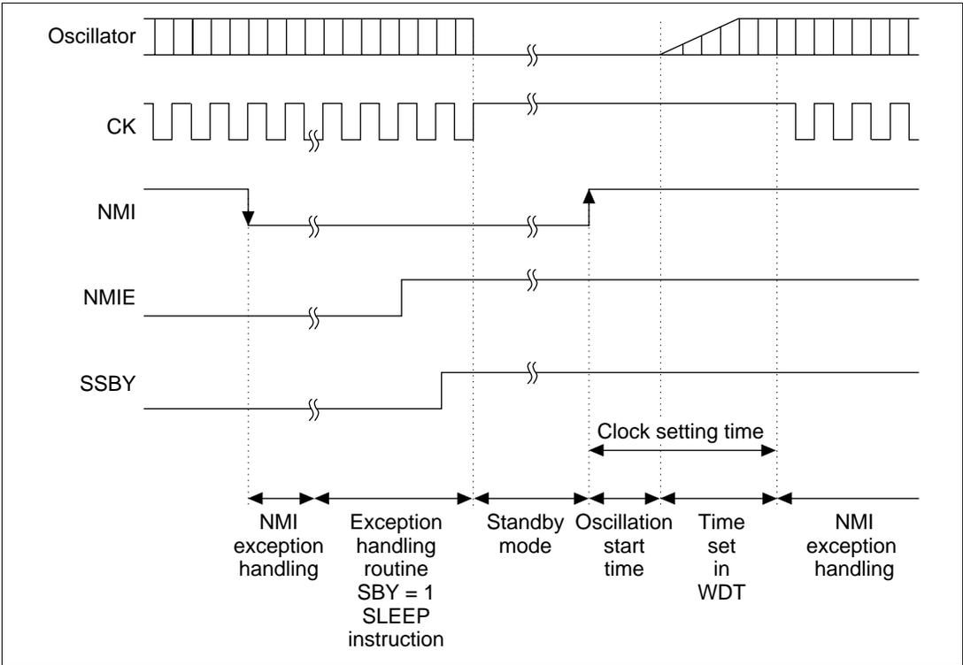
**Figure 19.1 NMI Timing for Standby Mode (Example)**
