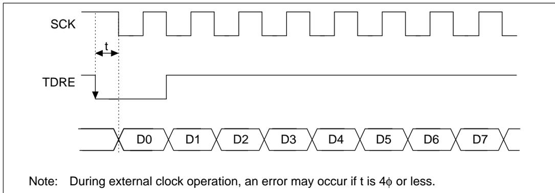
**Figure 13.22 Example of Synchronous Transmitting with DMAC**
