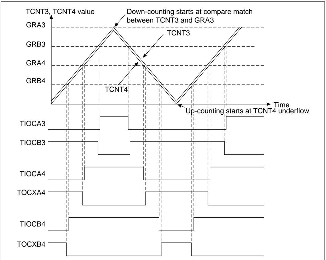
**Figure 10.34 Complementary PWM Mode Operation Example 1**
