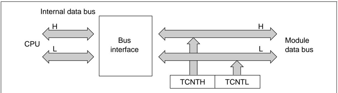
Figure 10.7 TCNT Access (TCNT to CPU (Word))
