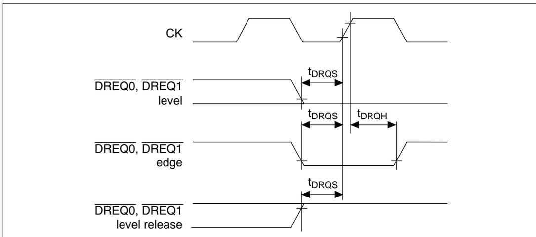
**Figure 20.65  $\overline{\text{DREQ0}}$ ,  $\overline{\text{DREQ1}}$  Input Timing (1)**
