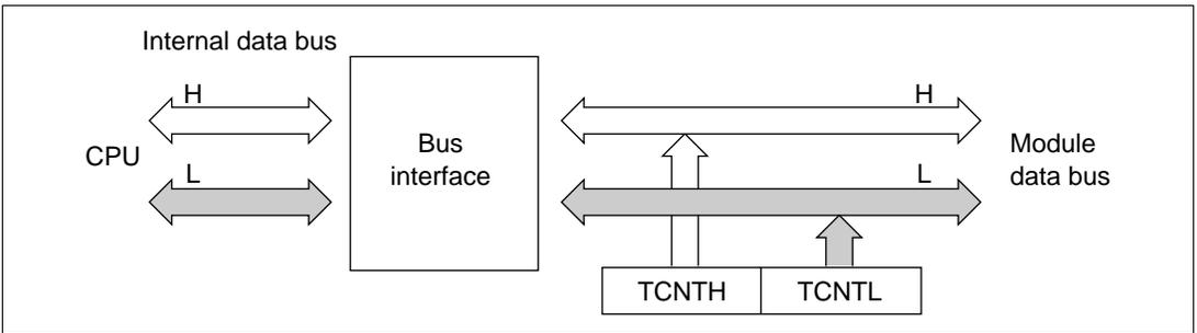
**Figure 10.11 TCNT Access (TCNT to CPU (Lower Byte))**
