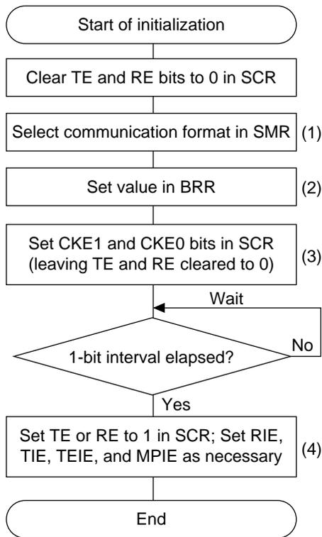
**Figure 13.4 Sample Flowchart for SCI Initialization**
