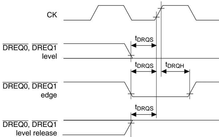
**Figure 20.34  $\overline{\text{DREQ0}}$ ,  $\overline{\text{DREQ1}}$  Input Timing (1)**
