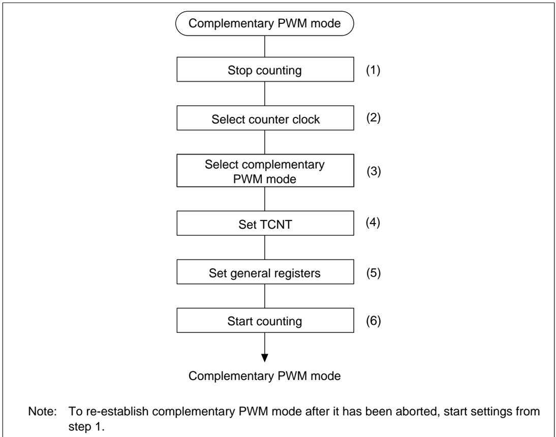
**Figure 10.33 Procedure for Selecting Complementary PWM Mode**
