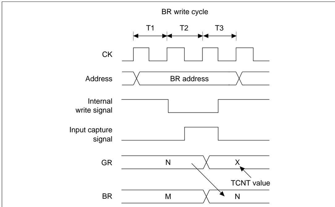
**Figure 10.66** Contention between BR Write and Input Capture
