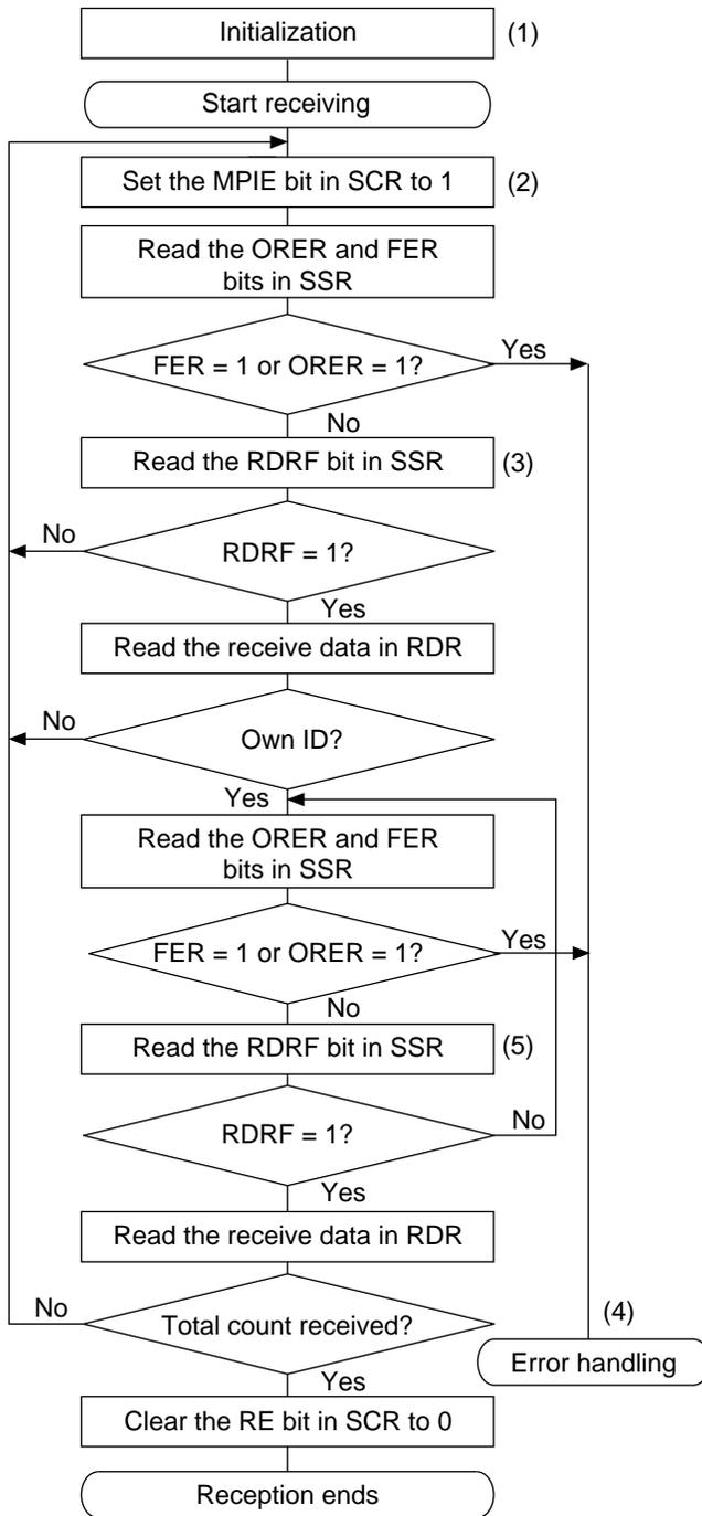
**Figure 13.12 Sample Flowchart for Receiving Multiprocessor Serial Data**
