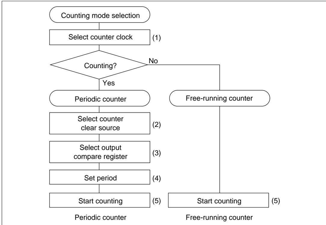
**Figure 10.14 Procedure for Selecting the Counting Mode**
