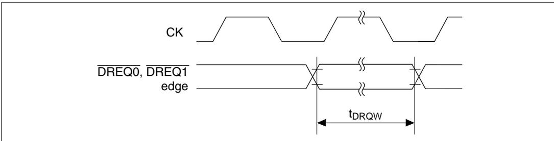
Figure 20.66  $\overline{\text{DREQ0}}$ ,  $\overline{\text{DREQ1}}$  Input Timing (2)
