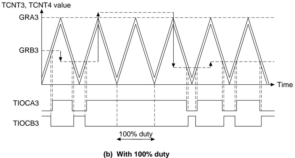
**Figure 10.35 Complementary PWM Mode Operation Example 2**
