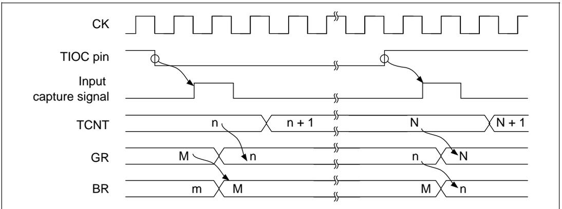
**Figure 10.51 Input Capture Timing Example for Buffer Operation**
