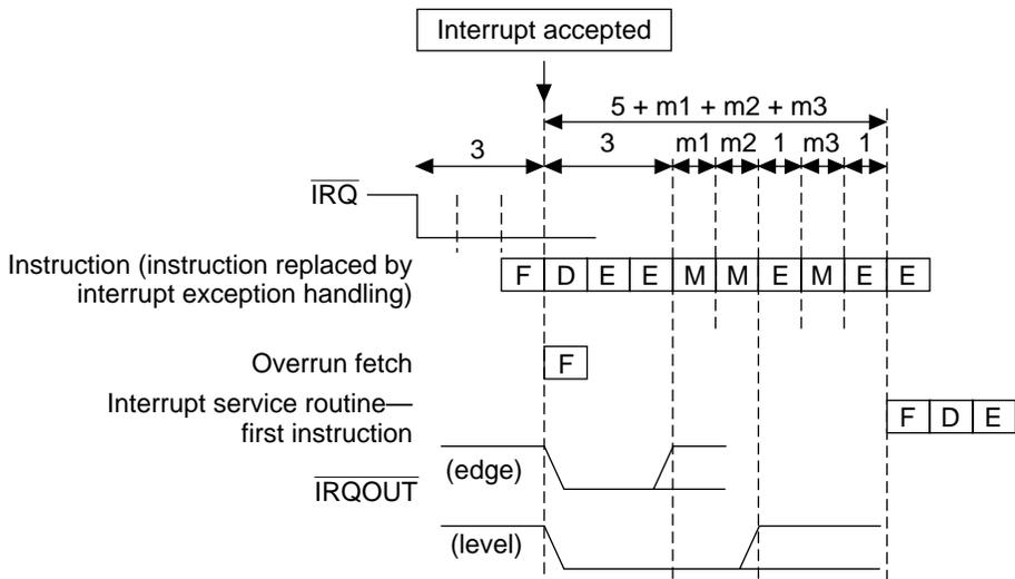
When  $m1 = m2 = m3$ , the interrupt response time is 11 cycles.
