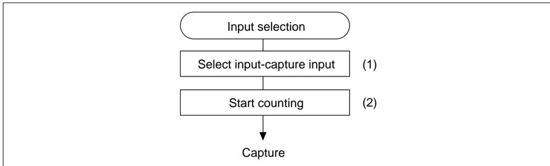
**Figure 10.23 Procedure for Selecting Input Capture Mode**
