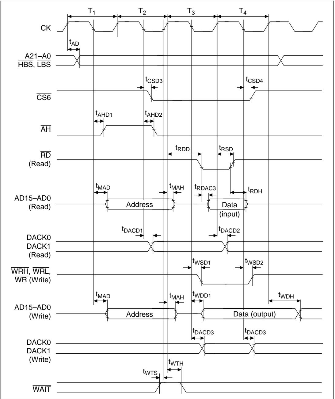
Figure 20.63 Address/Data Multiplexed I/O Bus Cycle
