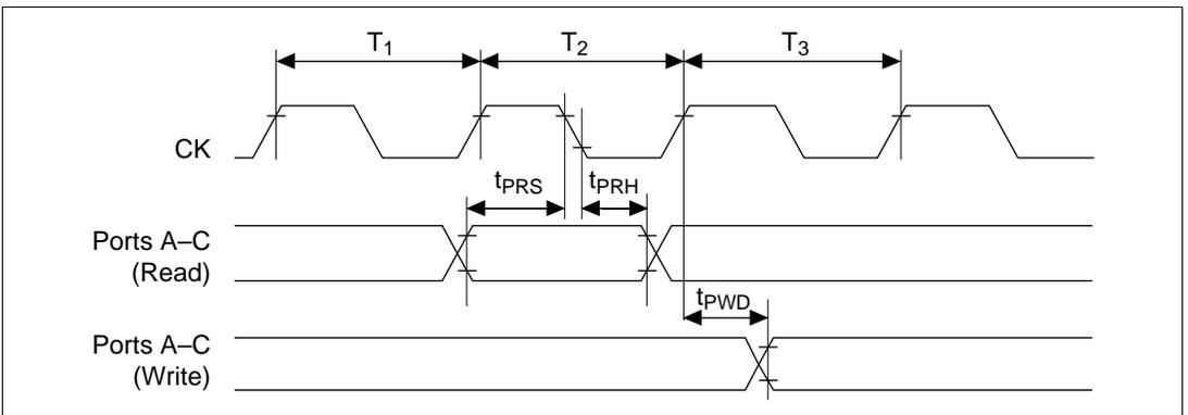
**Figure 20.69 Programmable Timing Pattern Controller Output Timing**
