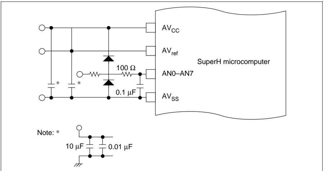
Figure 14.8 Example of Analog Input Protection Circuit
