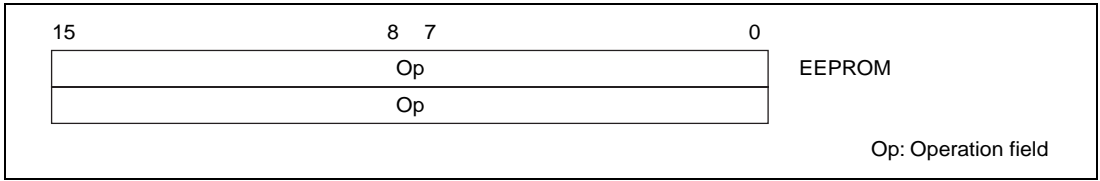
Figure 2.10 Block Data Transfer Instruction/EEPROM Write Operation Code
