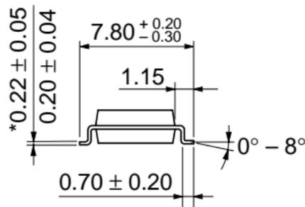
\*Dimension including the plating thickness
