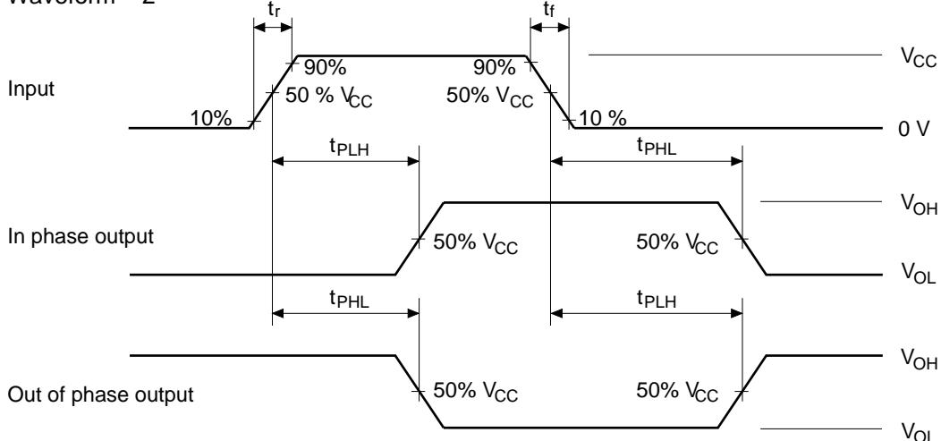
Notes: 1. Input waveform: PRR  $\leq$  1 MHz,  $Z_o = 50 \Omega$ ,  $t_r \leq 3$  ns,  $t_f \leq 3$  ns
