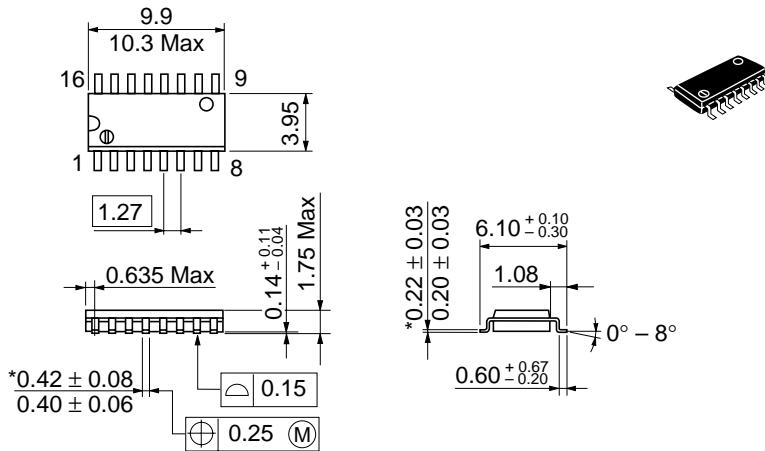
\*Dimension including the plating thickness
