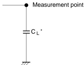
Note:  $C_L$  includes the probe and jig capacitance.
