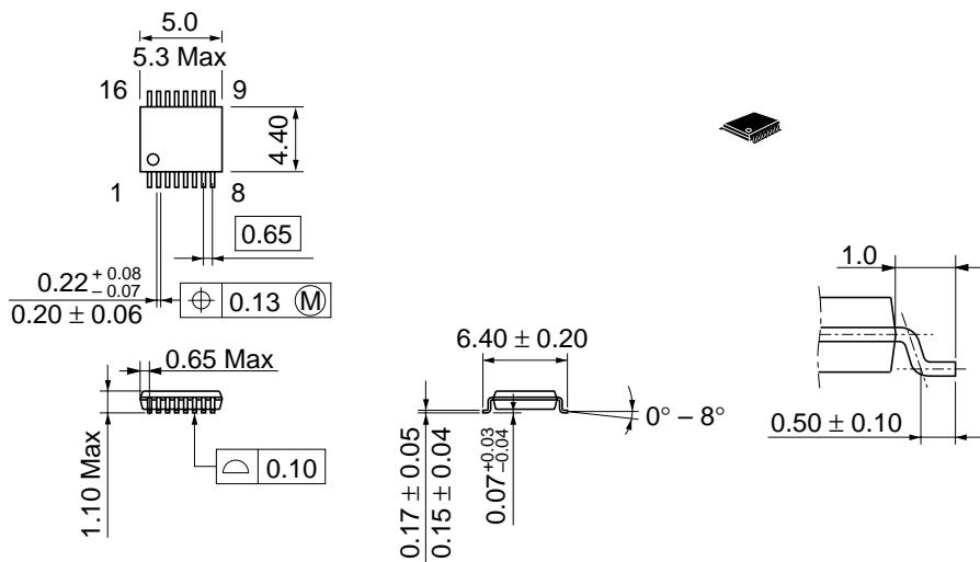
Dimension including the plating thickness
