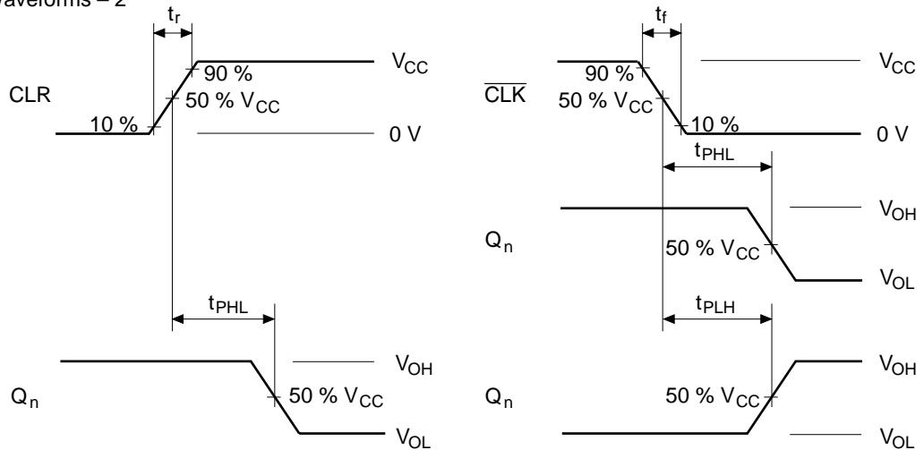
Notes: 1. Input waveform: PRR  $\leq$  10 MHz,  $Z_o = 50 \Omega$ ,  $t_r \leq 3$  ns,  $t_f \leq 3$  ns
