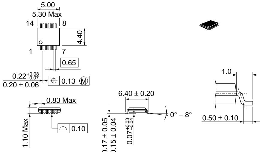
Dimension including the plating thickness
