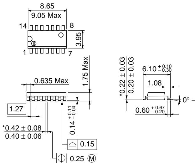
\*Dimension including the plating thickness
