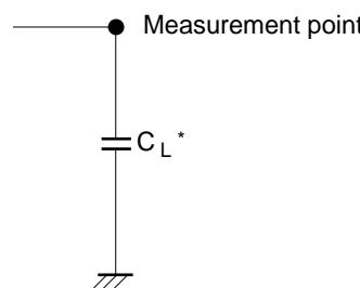
Note:  $C_L$  includes the probe and jig capacitance.
