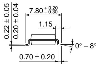
Dimension including the plating thickness
