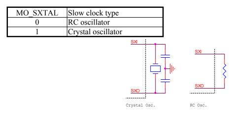
If the dual clock mode is used, the LCD display, Timer1 and Timer Base will derive its clock source from slow clock while the other blocks will operate with the fast clock.
