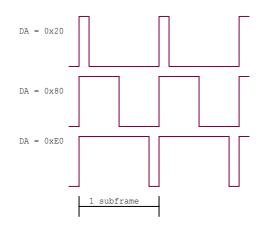
The PWM bit of VOC register controls register to enable the circuit and output driver. When PWM bit of VOC is '0', PWME bit and output drivers settings are both cleared. To use PWM for voice output, PWM bit has to be set to '1' first, then set PWME bit and enable output driver by setting the driver number. If PWM bit is disabled and enabled again, the setting for driver and PWME bit will be clear. V1.0E March 13, 2003 14
