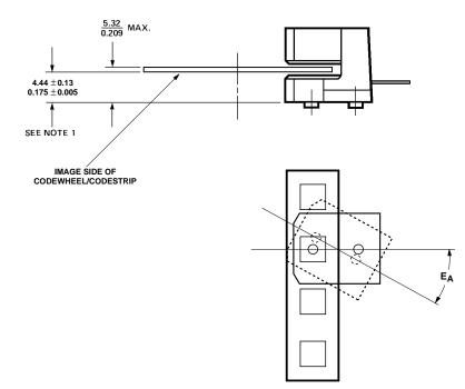
For linear motion, angular misalignment,  $\mathrm{E}_{\mathrm{A}}$  must be  $\leq~\pm~2$  degrees to achieve Encoding Characteristics.
