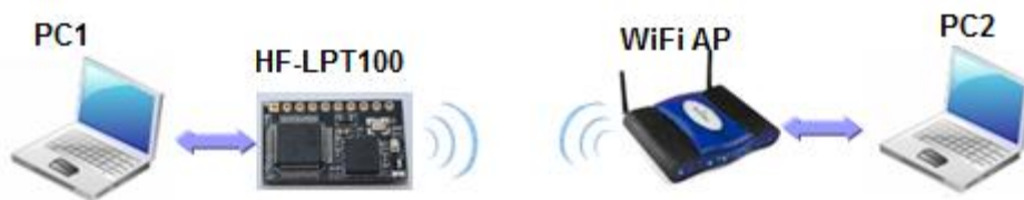
Figure 23. STA Interface Debug Connection
