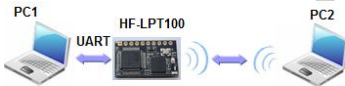
Figure 24. AP Interface Debug Connection
