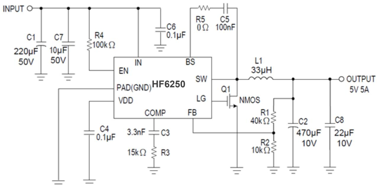
$V_{OUT} = V_{FB} \times (1 + R_1/R_2)$ ,  $V_{FB} = 1.00V$ ,  $R_2$  suggest  $10k\sim30k\Omega$
