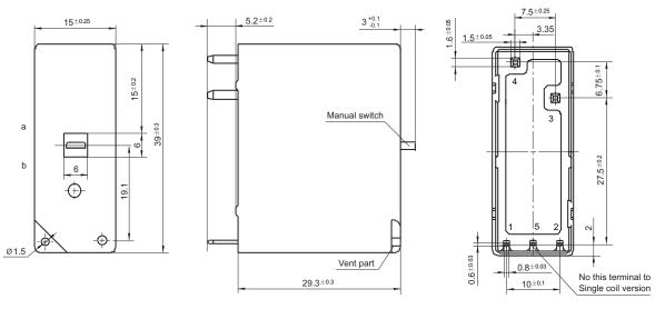
Remark: When the manual switch is pitched on point a, the contact is open; when the manual switch is pitched on point b, the contact is closed.
