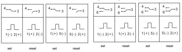
Single coil latching, 1 Form B Double coils latching, 1 FormB
