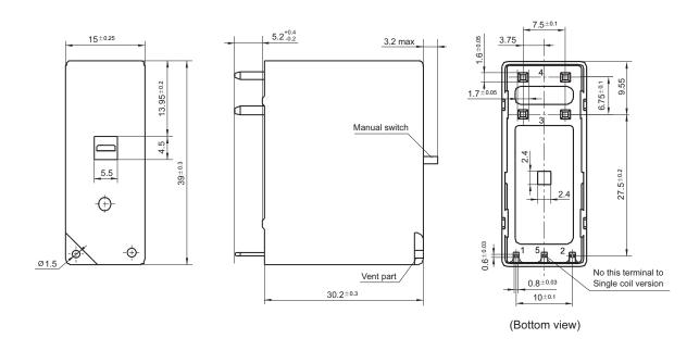
Remark: In case of no tolerance shown in outline dimension: outline dimension  $\leq$ 1mm, tolerance should be  $\pm$ 0.2mm; outline dimension >1mm and  $\leq$ 5mm, tolerance should be  $\pm$ 0.3mm; outline dimension >5mm, tolerance should be  $\pm$ 0.4mm.
