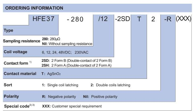
Notes: 1) 2SH means that relay is on the "reset" status when delivery; 2SD means that relay is on the "set" status when delivery. If no speical
