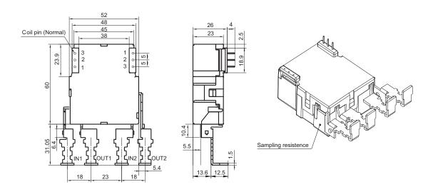
Remark: In case of no tolerance shown in outline dimension: outline dimension ≤1mm, tolerance should be ±0.2mm; outline dimension >1mm and ≤5mm, tolerance should be ±0.4mm; outline dimension >5mm, tolerance should be ±0.4mm.
