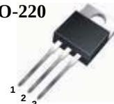
1.Gate 2. Drain 3. Source
