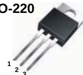
1.Gate 2. Drain 3. Source
