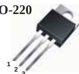
1.Gate 2. Drain 3. Source
