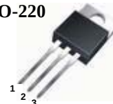
1. Gate 2. Drain 3. Source
