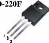
1. Gate 2. Drain 3. Source
