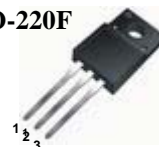
1.Gate 2. Drain 3. Source
