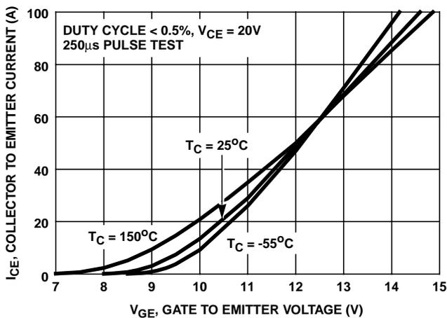
FIGURE 13. TRANSFER CHARACTERISTIC
