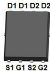
DFN5X6-8L top view
