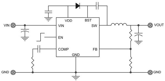
Note: When using a solid or ceramic input Cap, It is recommended to parallel a TVS diode.
