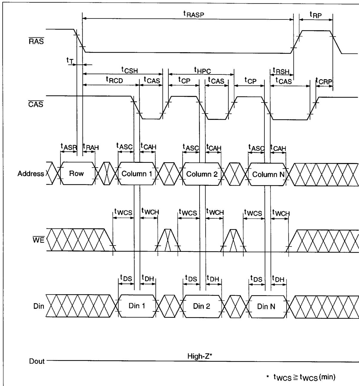
**EDO Page Mode Delayed Write Cycle<sup>18</sup>**
