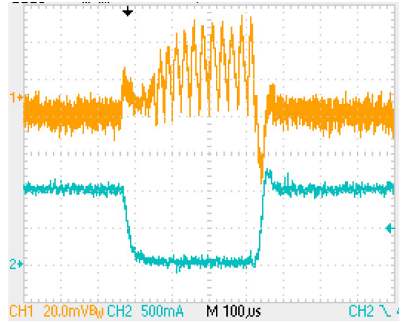
Buck Load Transient Response (Ibuck=100mA to 600mA, VBAT=3.6V, Vbuck=1.2V, Cout=4.7uF)
