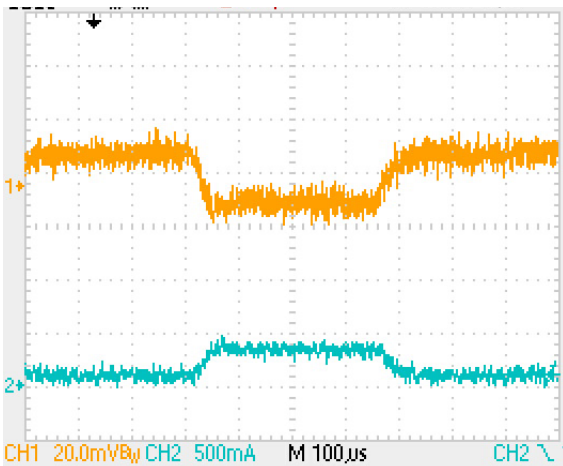
LDO1 Load Transient Response (ILDO1=50mA to 200mA, VBAT=3.6V, Cldo1_out=1uF)
