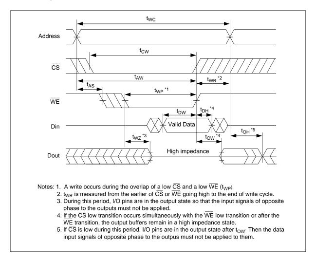
Write Timing Waveform (1) (WE Controlled)
