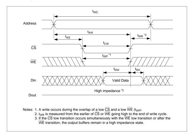
Write Timing Waveform (2) ( $\overline{\text{CS}}$  Controlled)
