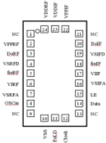
Leadless Grid Array Package
