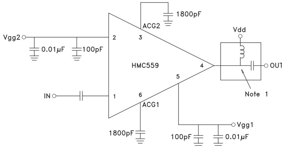
**NOTE 1:** Drain Bias (V<sub>dd</sub>) must be applied through a broadband bias tee with low series resistance and capable of providing 500mA
