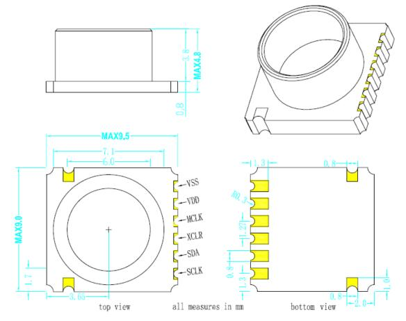
HP03 Series of calibrated sensor module HP03S
