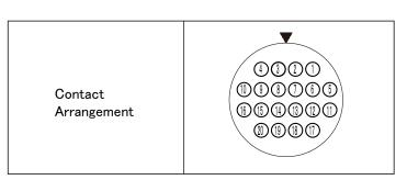
In the figure above, the mark ▼ indicates the position of the main mating guide
