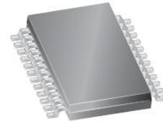
TSSOP28 with exposed thermal pad
