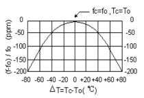
The curve shown above accounts for resonator contribution only and does not include oscillator temperature characteristics.
