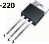
1.Gate 2. Drain 3. Source
