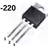
1.Gate 2. Drain 3. Source
