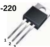
1.Gate 2. Drain 3. Source
