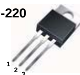
1.Gate 2. Drain 3. Source
