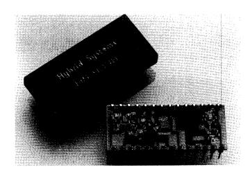
ter. In addition to these input functions are two chip select inputs and a read/write input allowing direct memorymap configurations. All input controls are static to allow hardwired configurations. The DAC338 is packaged in a hermetically sealed package and is rated -55°C to +125°C. The B-models of the DAC338 are fully screened and tested to MIL-STD-883 Rev. C, Level B requirements.
