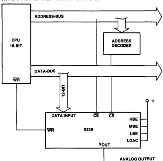
Interfacing the HS9338 to a 16-Bit microprocessor is quite easy, because no multiplexing of the data inputs is necessary. An address decoder and the second chip-select input is used to select the DAC.
