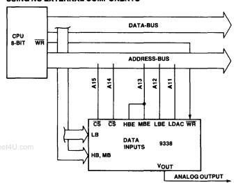
This mode of operation requires 13k bytes of unused addresses. No additional address decoder is necessary. The two chip-select inputs together with the byte-enable and load-DAC inputs are used to control all functions of the DAC. Through selecting the address-lines the user can vary the addresses used to control the DAC. In the above figure the control signals have the following address-configurations (hex):
