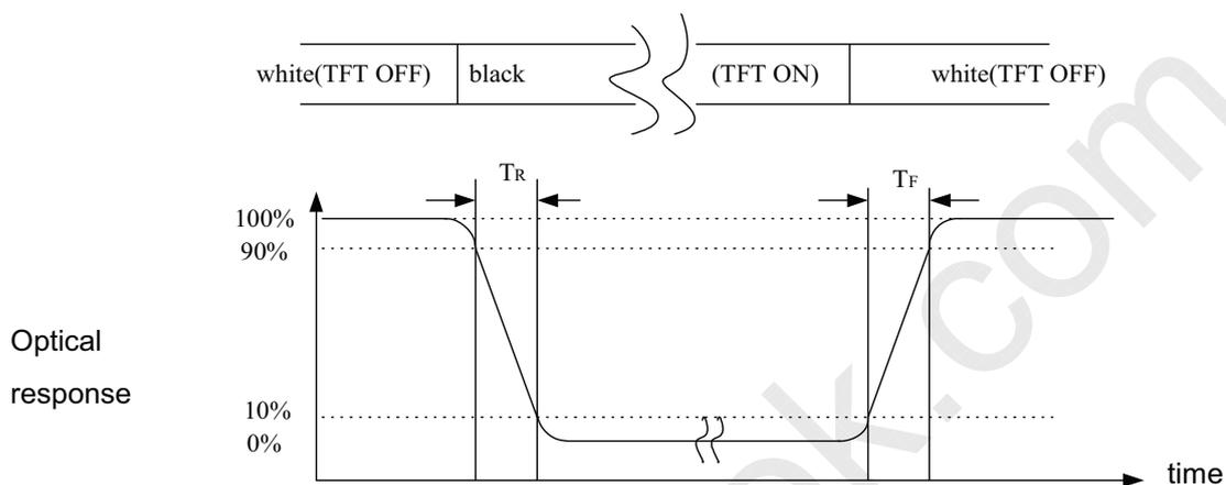
Note (4) Optical characteristic measurement setup
