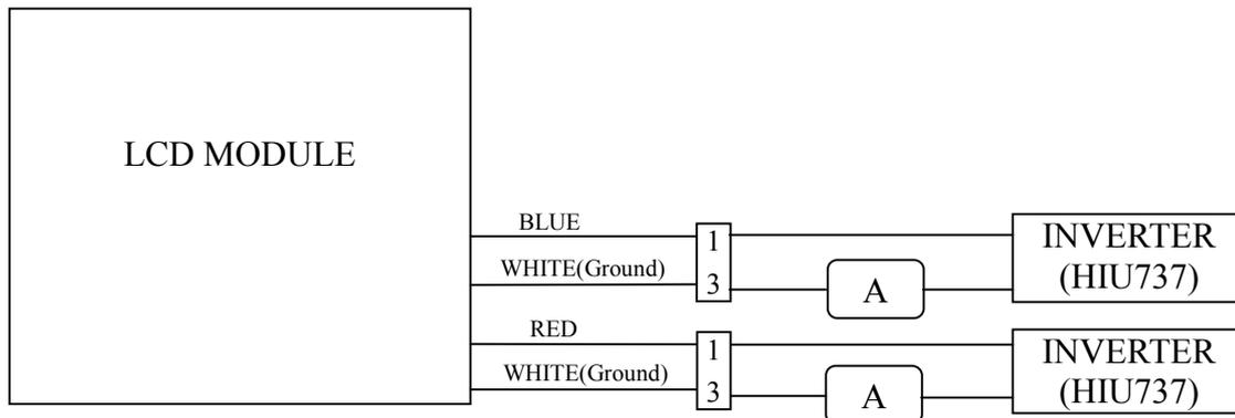
(2)Lamp frequency may produce interference with horizontal synchronous frequency and this may cause line flow on the display. Therefore lamp frequency shall be detached from the horizontal synchronous frequency and its harmonics as far as possible in order to avoid interference.
