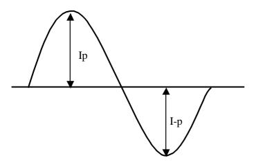
Asymmetry rate =  $|I_p-I_{-p}| / I_{rms} x 100\%$ Distortion rate =  $I_p$  (or  $I_{-p}$ ) /  $I_{rms}$
