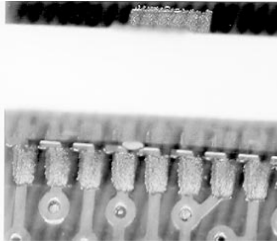
Photo 1.0. Castellations misaligned to land pads in x-axis before reflow.
