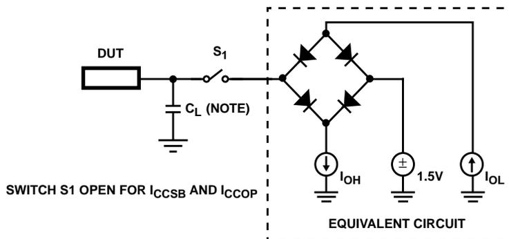
NOTE: Test head capacitance.
