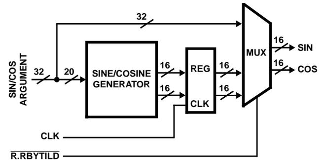
FIGURE 2. SINE/COSINE SECTION
