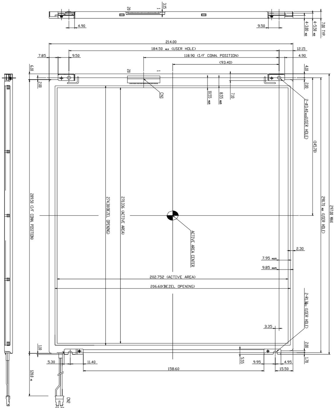
**Figure 6. TFT-LCD Module Outline Dimensions (Rear view)**
