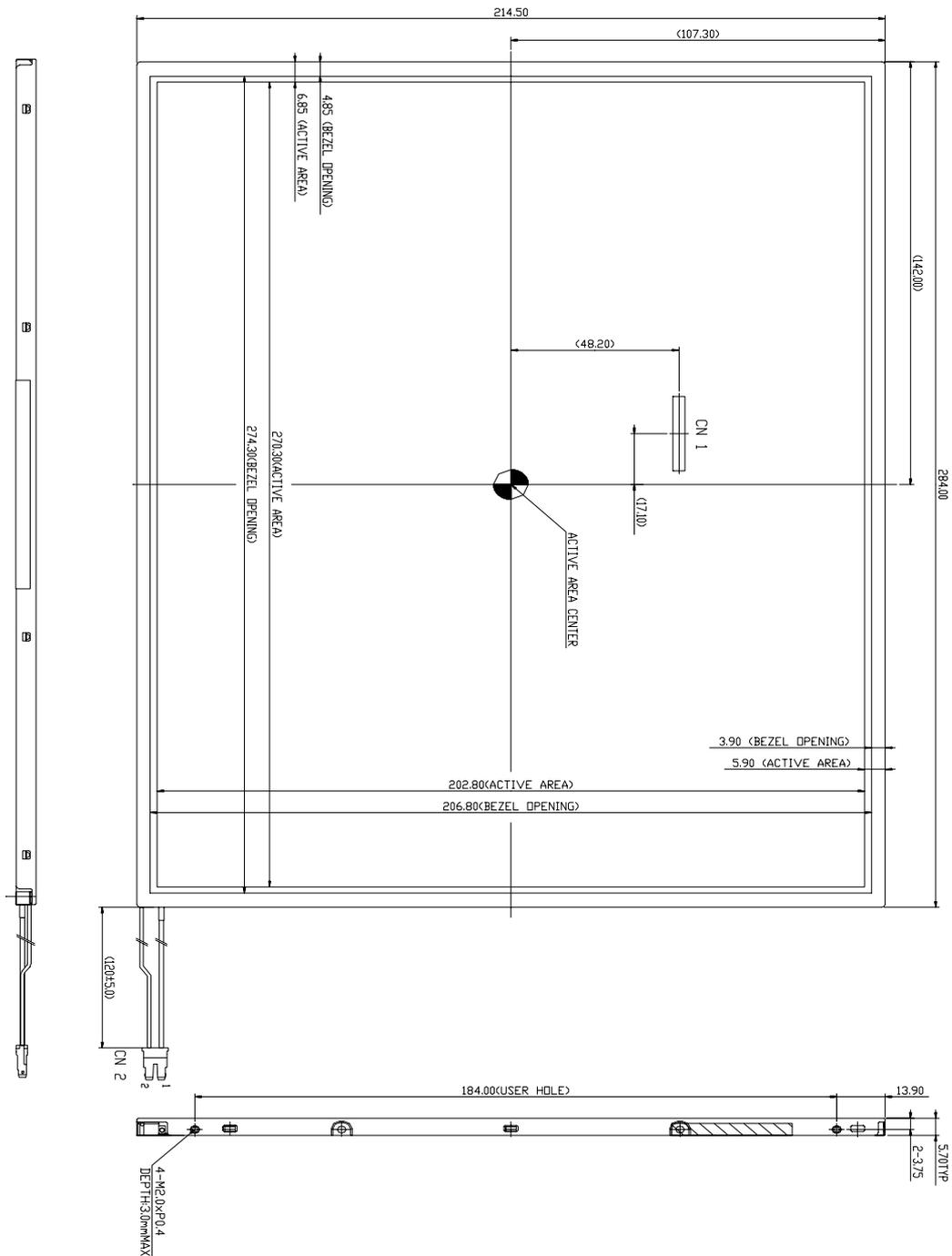
Figure 6. TFT-LCD Module Outline Dimensions (Rear view)
